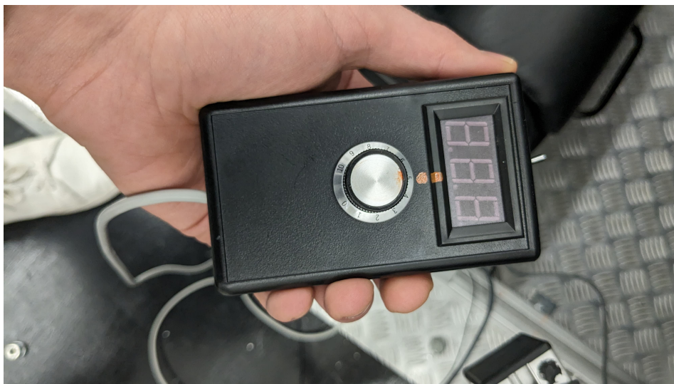
Figure 4.6: The Comfort Knob. A marking was made on the neutral position, and a figure was placed in the screen to help the participant remember which way to turn the knob.
