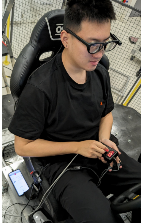
Figure 4.4: One of the participants in full setup. In the picture the eye tracking glasses are on his head, connected to the phone that can be seen in the bottom left. The phone is held in place using velcro tape. In his hand, the participant is operating the comfort knob. on his left index and middle finger, the velcro straps with GSR electrodes are attached. The GSR electrodes and heart rate electrodes, which are under the participants' shirt, are connected to the grey/black NeXus device next to the phone. This device is also held in place using velcro tape.
