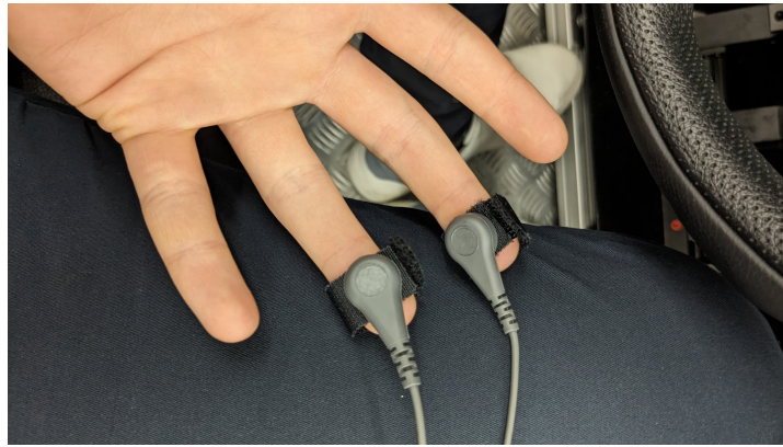
Figure 4.8: The velcro straps with GSR sensors attached to the fingertips of the non-dominant hand. They are not color-coded because it does not matter which goes on which finger, as long as they are on the same hand.
