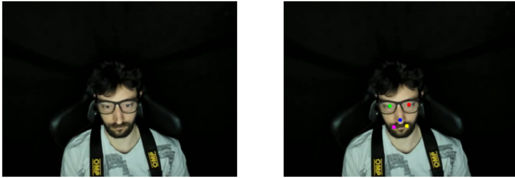
Figure 3.6: Capture from the webcam during the experiment, with the left image showing the raw footage, and the right image showing the facial landmarks detected by RetinaFace.
