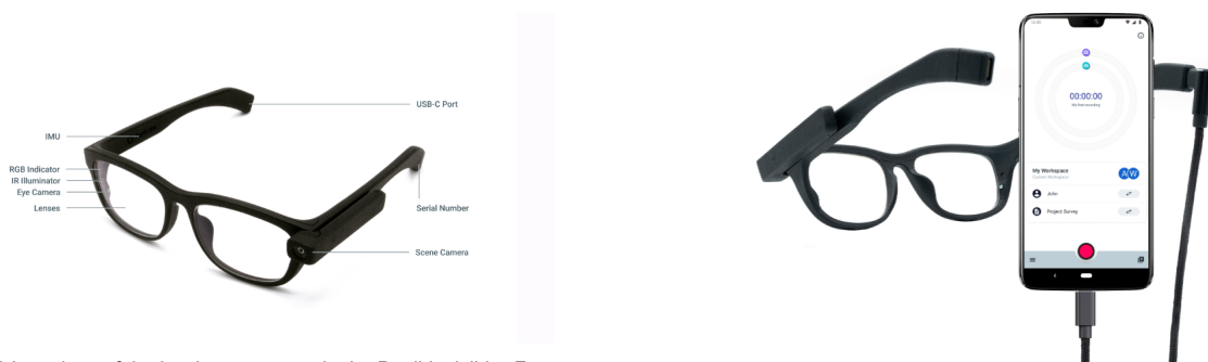
(b) The Pupil Invisible glasses come with a smartphone with their own software application on it. Measurements are set-up and started from this phone.
