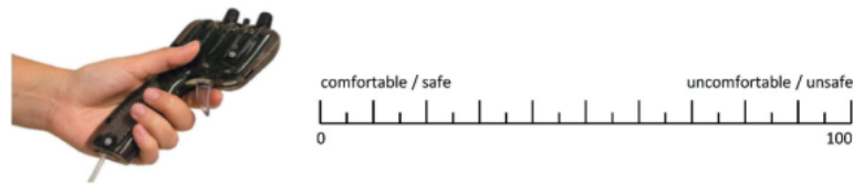
Figure 2.7: Handset control and the corresponding response scale, used to continuously assess perceived discomfort during an automated drive (Beggiato, Hartwich, et al., 2020).
