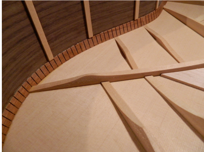
Figure 2: Close-up of the braces attached to the top plate.
