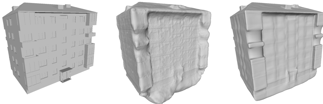
Figure A.1.: Left ground truth mesh, middle NeuS-facto output, right VolSDF output for the apartment model
