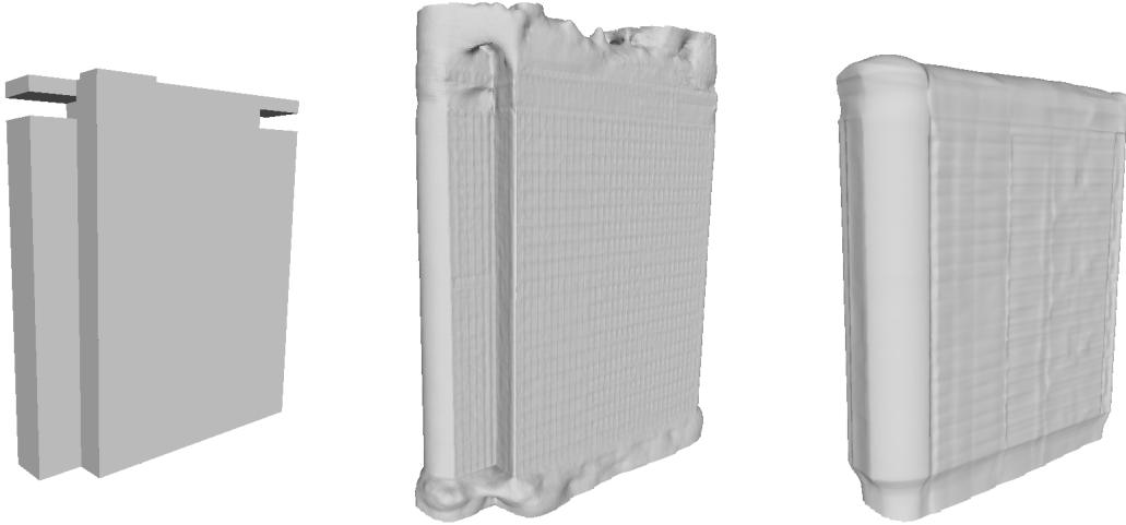
Figure A.2.: Left ground truth mesh, middle NeuS-facto output, right VolSDF output for the Ewi model
