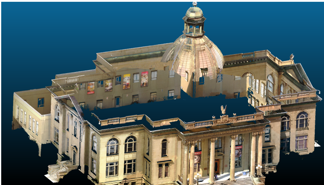
Figure 2.4.: The courthouse objects misses a lot of data especially for the roof
