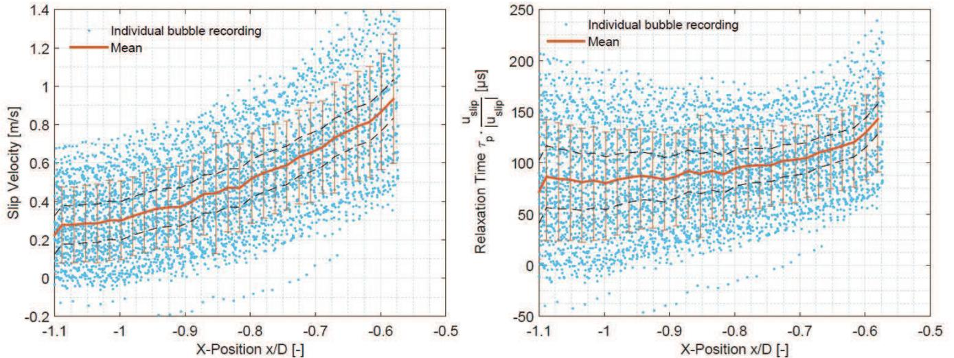
**Fig. 4** Slip velocity (left) and relaxation time (right) of individual bubbles on the stagnation line of the cylinder for heavier-than-air air-filled soap bubbles. Black dashed lines indicate the uncertainty due to the freestream turbulence intensity.
