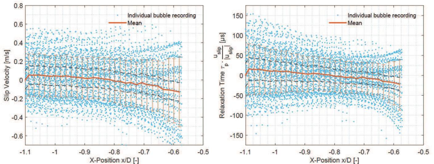
**Fig. 5** Slip velocity (left) and relaxation time (right) of individual bubbles on the stagnation line of the cylinder for neutrally buoyant helium-filled soap bubbles. Black dashed lines indicate the uncertainty due to the freestream turbulence intensity.
