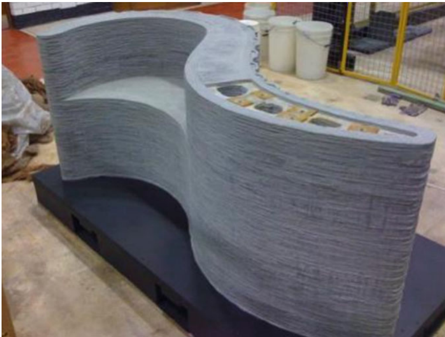
Fig. 6.9 Digital manufacturing of a free-shaped wall-like concrete bench (Buswell et al. 2018)
