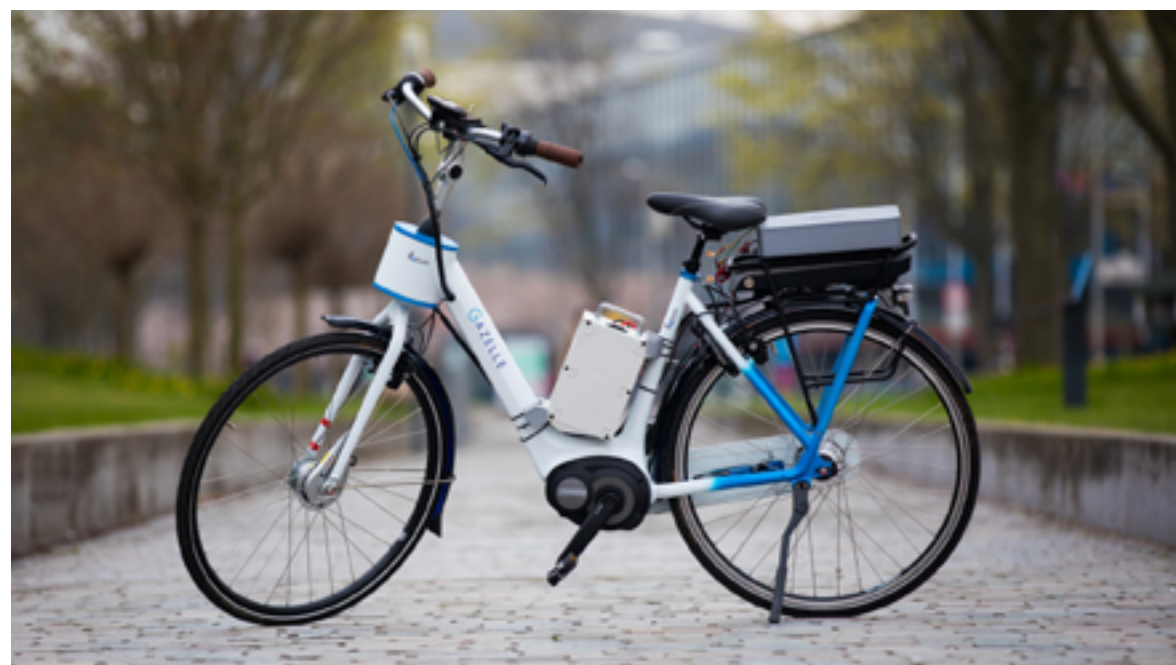
Figure 17. Self-balancing bike (TU Delft, 2019)
