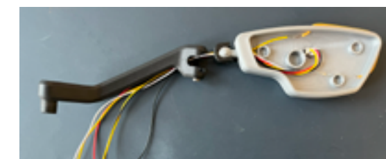
Figure 54. Printed model of mirror with LED installed
