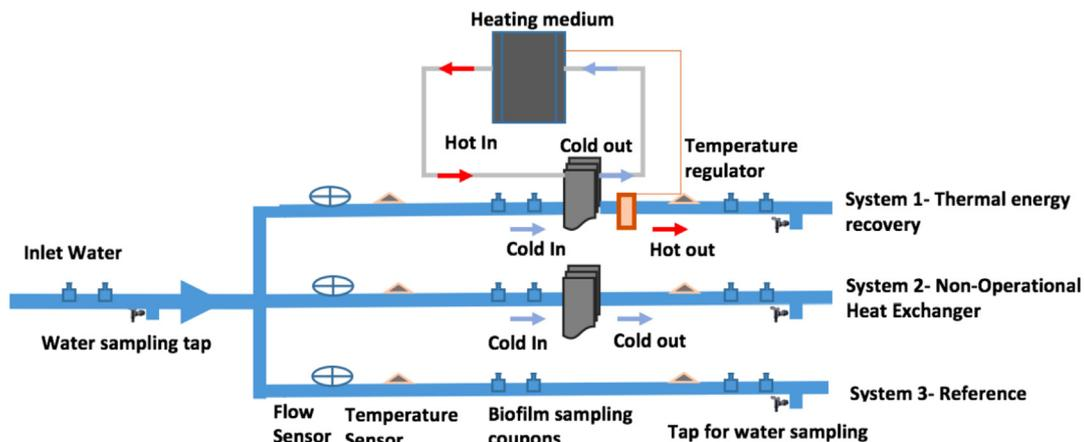
Fig. 4. Laboratory scale drinking water distribution systems.
