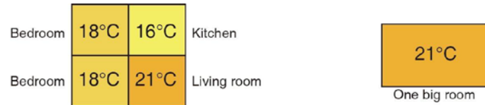
Fig 4 Difference of design temperature between a conventional apartment and single-living studio
