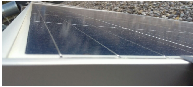
Figure 5.1: Dust in the PV module due to the natural accumulation for 8 days period.
