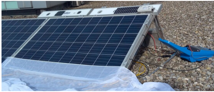
Figure 2.19: Placing of white fabric to simulate non-uniform soiling at T_{loss} of 30%.
