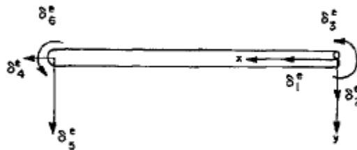
2.10 Cable element with 6 d.o.f.
