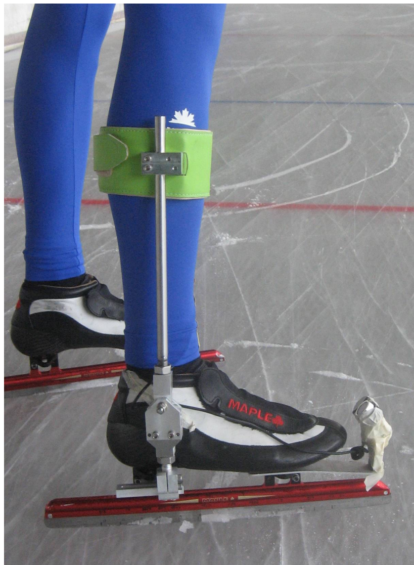
Figure 12. Total view of the orthosis. The height of the green brace along the bar can be adjusted as can the location of the rotation axis
