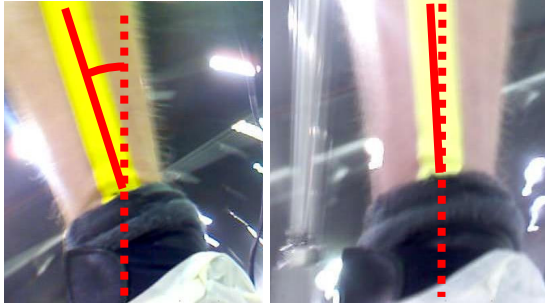
Figure 17. Images from the camera on the skate. Both depict the maximum ankle eversion angle (MAX \alpha_{AE} ) during a stroke. The \alpha_{AE} is the angle between the full line and the dotted line. In the left image with normal ankle eversion the \alpha_{AE} is 17 degrees. In the right with reduced ankle eversion image the \alpha_{AE} is 4 degrees.
