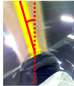
Figure 14. Image from the camera on the skate. The ankle eversion angle ( \alpha_{\text{AE}} ) is the angle between the vertical line of the recording (dotted line) and the yellow strip along the tibia.
