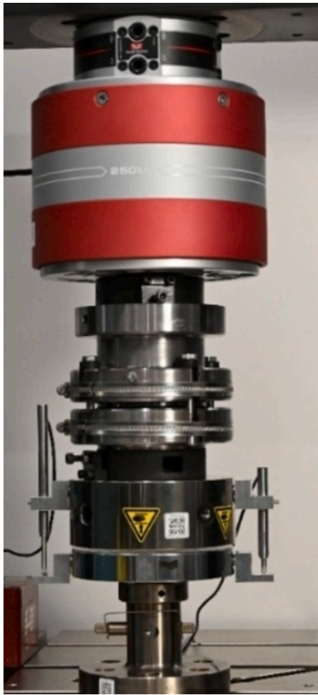
Fig. 2. Example compression test setup including lockable self-aligning platen and LVDTs.
