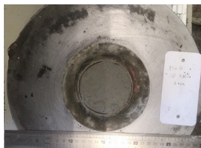
(b) Top view of Slump Flow Table test prior to testing
