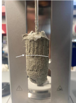
Figure 8.19: D-PVA8 specimen that failed on shear during testing at the age of 10 minutes
