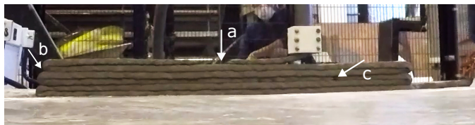
Figure 4.1: Filament breakage indicated with (a) and printing irregularities (b & c) during printing at TUE
