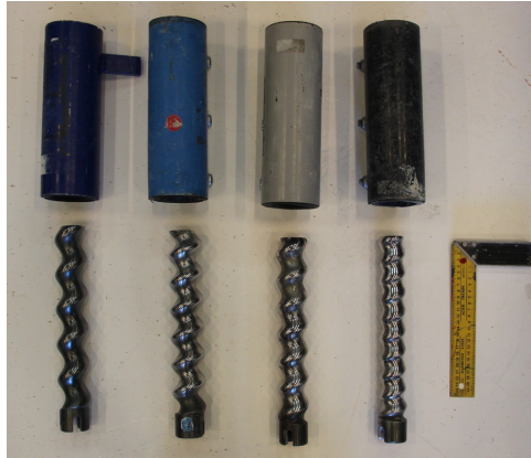
Figure 4.7: The selection of rotors/stators that were assessed, from left to right: D8-2, D7-2.5, D4-1/2, D4-1/4
