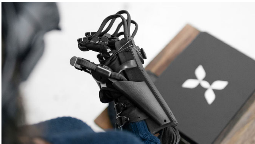
Fig. 23: Haptic glove with pressure points and force feedback
