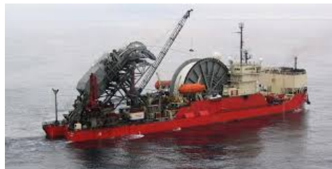
(c) Pipe laying vessel
