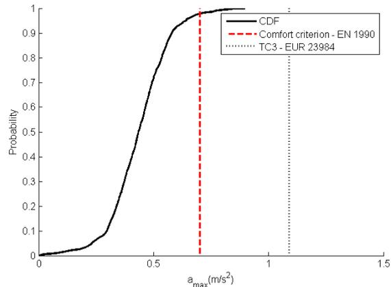
Figure 11.38: Cumulative density function of the maximum accelerations per single pedestrian crossing the bridge within a crowd density of  $0.5 \text{ P/m}^2$ , compared with the maximum acceleration calculated with EUR 23984 for the bridge  $L = 50 \text{ m}$
