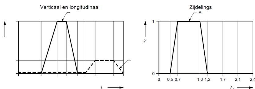
Figure 4.1: Reduction coefficient  $\psi$  according to the Eurocode [5]
