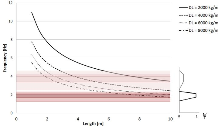
Figure 6.2: Relation between natural frequency and length of a cantilever footbridge with different dead load with critical frequency range for pedestrians
