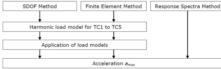
Figure 4.6: Methods for calculating the maximum acceleration [6]
