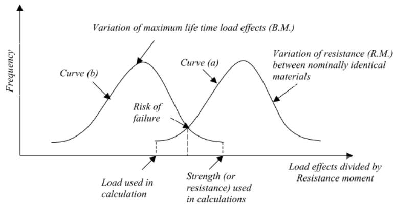
Figure 3.8: Risk of failure of a structure [20]
