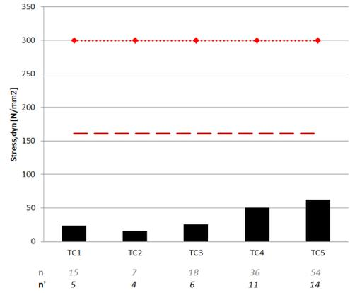
Figure 6.8: Stresses for beam L = 12 m
