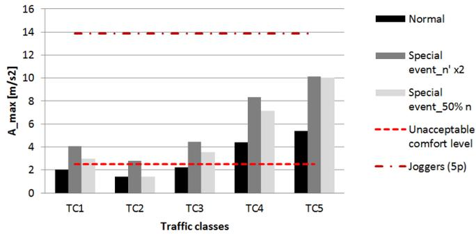
Figure 6.15: Accelerations for a bridge L = 12m
