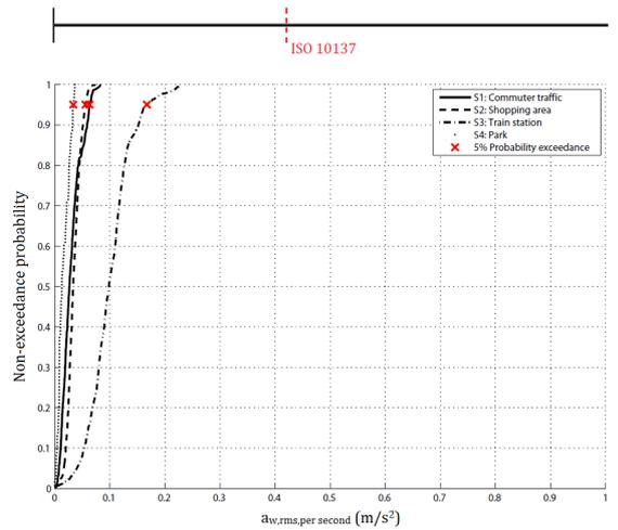
Figure 12.28: Cumulative density functions of the expected r.m.s. per second of the weighted accelerations per single pedestrian for the scenarios based on group formation and  $L = 100$  m
