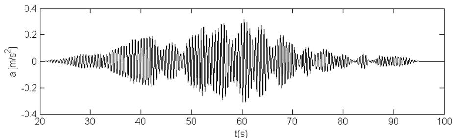
Figure 11.33: Example of a typical acceleration signal which a single individual pedestrian perceives crossing a footbridge with  $L = 100 \text{ m}$
