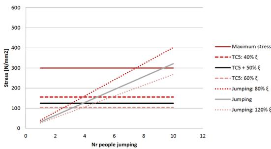
Figure 6.21: Stresses for a bridge L = 12 m
