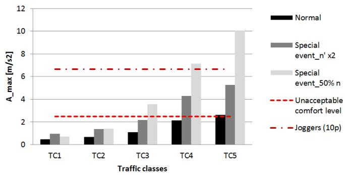
Figure 6.17: Accelerations for a bridge L = 50m
