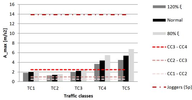
Figure 6.29: Accelerations for a bridge L = 12 m with different damping properties
