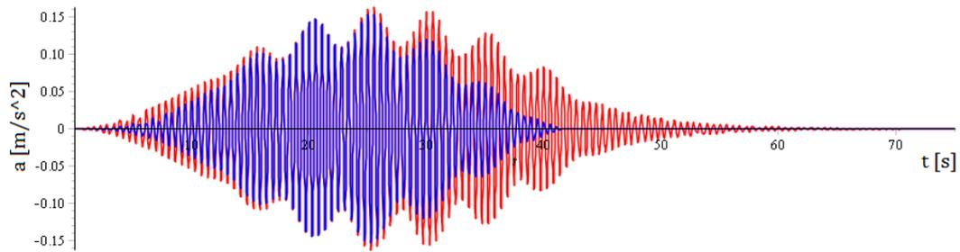
Figure D.12: Acceleration of the bridge (red) due to two separate pedestrians for the first mode at  $x = 25$  m and the accelerations the first pedestrian experiences (blue) when crossing the bridge - Maple
