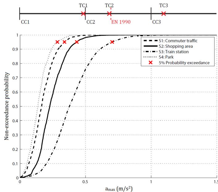
Figure 11.39: Cumulative density functions of the maximum expected accelerations per single pedestrian for the four scenarios based on densities and  $L = 50 \text{ m}$
