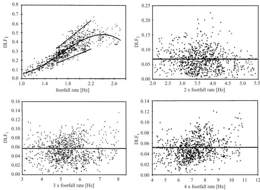
Figure 3.2: DLFs of the walking force for the first four harmonics after Kerr [13]
