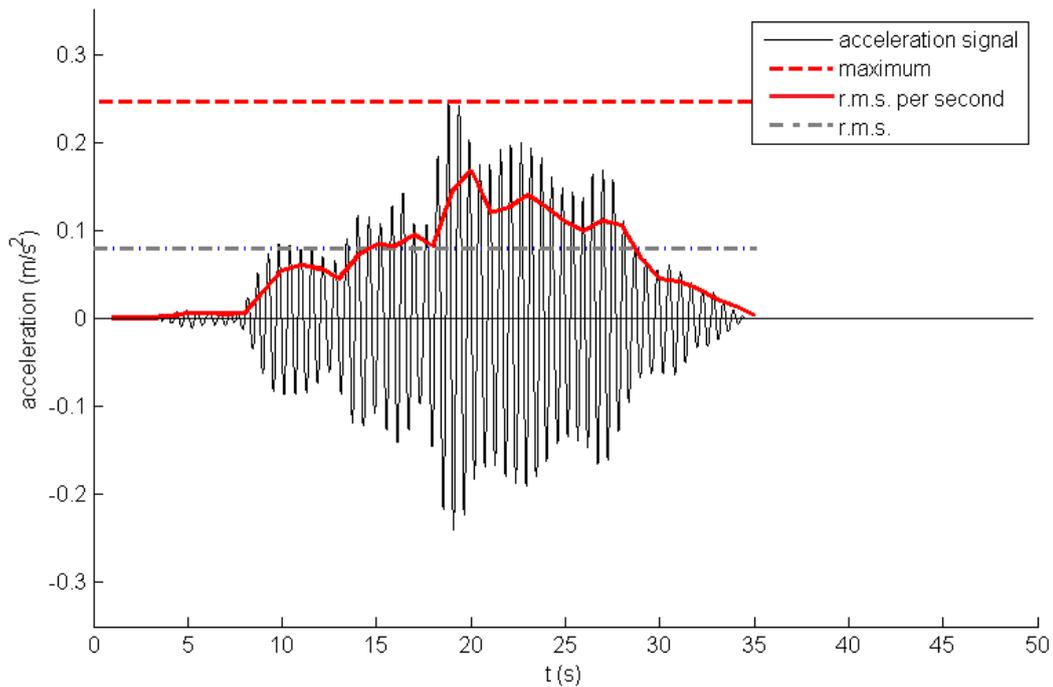
Figure 11.36: Evaluated acceleration signal for one pedestrian crossing a bridge with  $L = 50$  m within a crowd with a density of  $0.5 \text{ P/m}^2$
