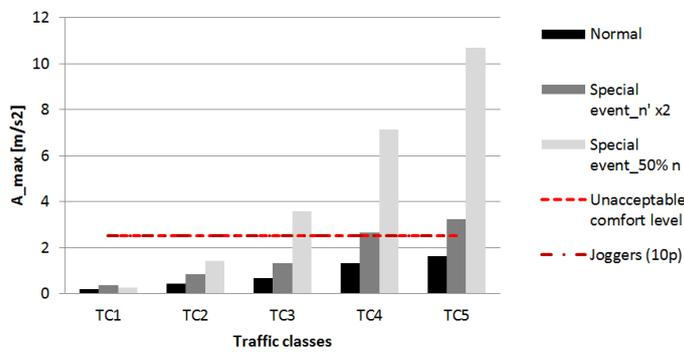
Figure 6.19: Accelerations for a bridge L = 100m
