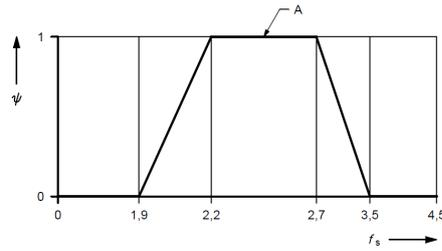
Figure 4.2: Reduction coefficient  $\psi$  for a single jogger [5]
