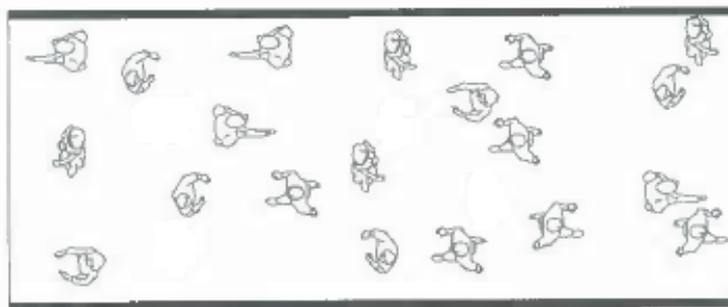
Figure 10.3: Pedestrian density of 0,5 P/m<sup>2</sup> based on a figure with different pedestrian densities presented by Schlaich [64]
