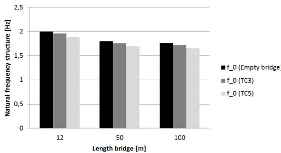
Figure 6.37: Change in frequency by taking into account additional mass due to pedestrians
