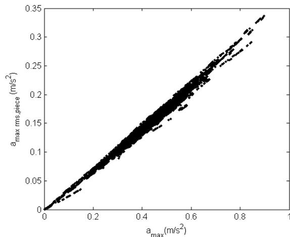
Figure 12.16: The correlation between the maximum acceleration and the maximum of the r.m.s. per second of the acceleration per single pedestrian for a bridge  $L = 50$  m and a traffic density of  $0.5 P/m^2$
