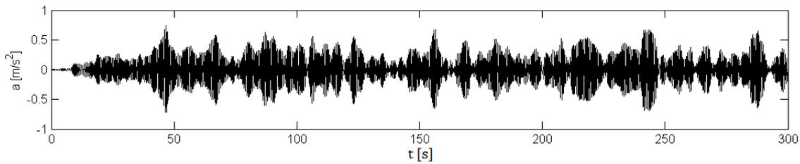
Figure 11.29: Example of the accelerations of the bridge with  $L = 50 \text{ m}$  for a crowd with a density  $0.5 \text{ P/m}^2$  for the first mode shape (at mid span:  $L = 25 \text{ m}$ )
