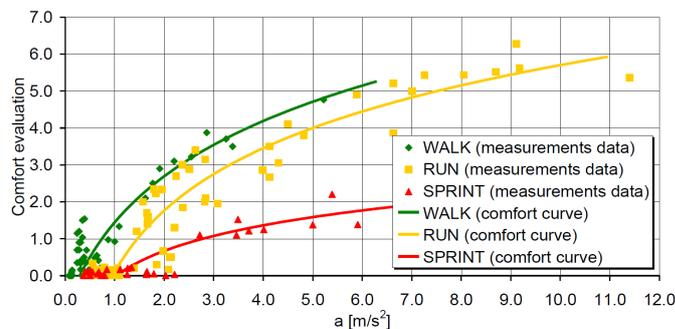
Figure 10.13: Comfort curves and areas, adjusted based on survey data by Hawryszków [16]
