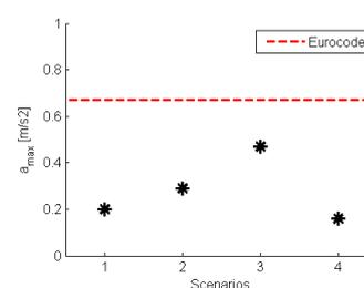
Figure 12.8: Results of the maximum accelerations for the four scenarios based on densities for L = 100m
