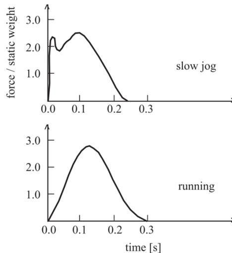
Figure 3.4: Typical vertical force patterns in relation to the static weight for slow jogging and running [10]
