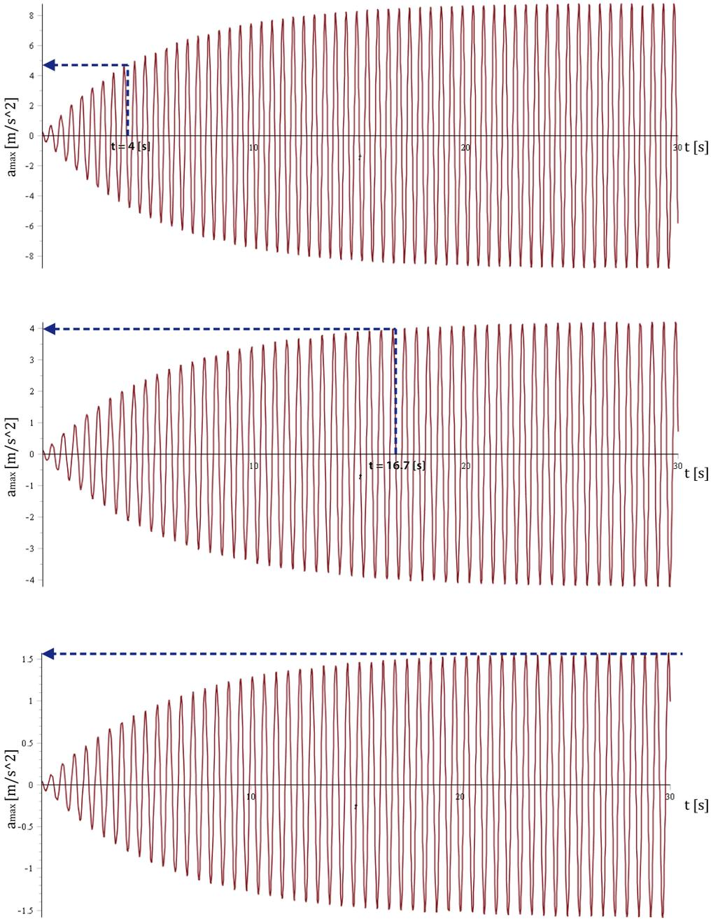
Figure C.2: Response in acceleration of the bridge deck by joggers from top to bottom  $L = 12, 50$  and  $100$  m
