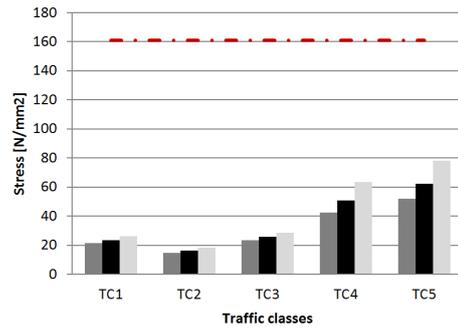
Figure 6.30: Stresses for a bridge L = 12 m with different damping properties
