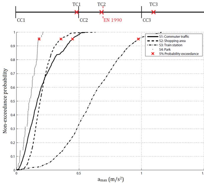
Figure 11.40: Cumulative density functions of the maximum expected accelerations per single pedestrian for the four scenarios based on group formation and  $L = 50$  m
