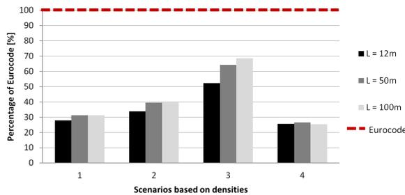
Figure 12.12: Comparison of the results of the accelerations for the scenarios based on densities with the expected bridge acceleration of the Eurocode - expressed in percentage [%] of the Eurocode acceleration
