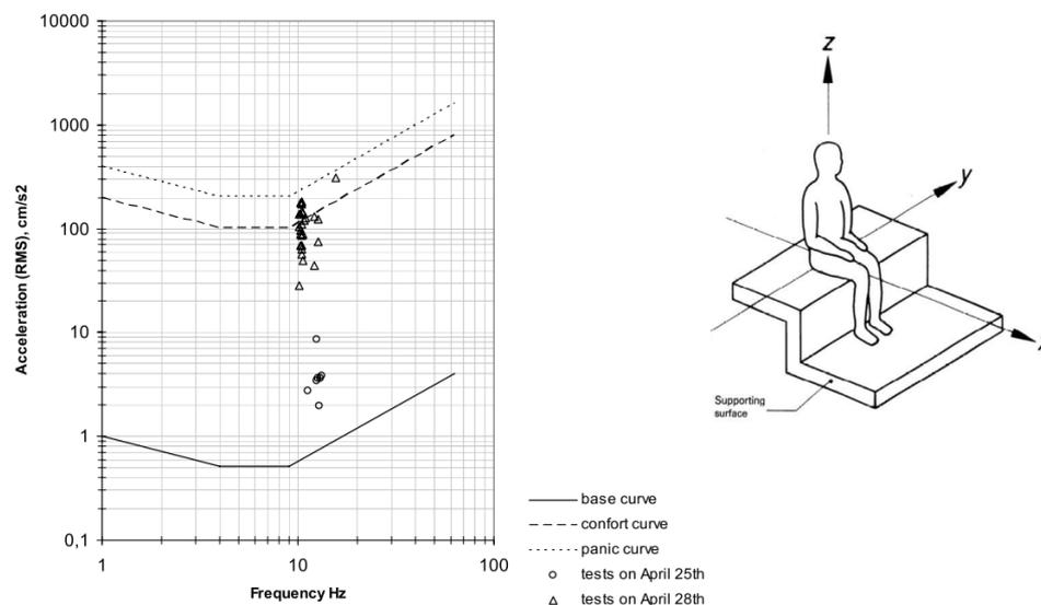
Figure 10.2: Vibration z-axis limits curve for acceleration (foot-to-head direction) and test values for grandstands by Marques [63]
