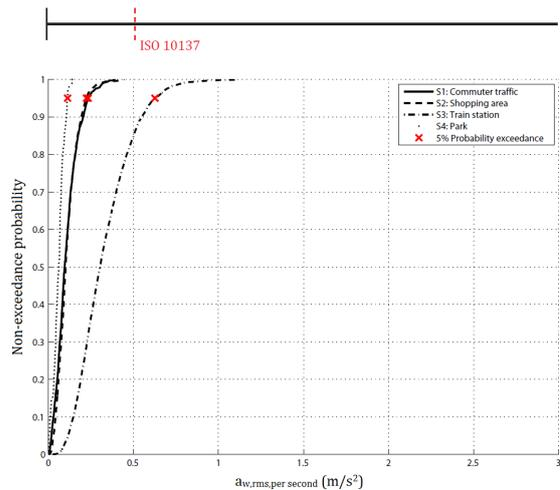
Figure 12.24: Cumulative density functions of the expected r.m.s. per second of the weighted accelerations per single pedestrian for the scenarios based on group formation and L = 12 m
