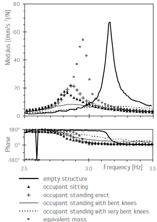
Figure 5.14: FRFs of an empty and occupied concrete plank [50]
