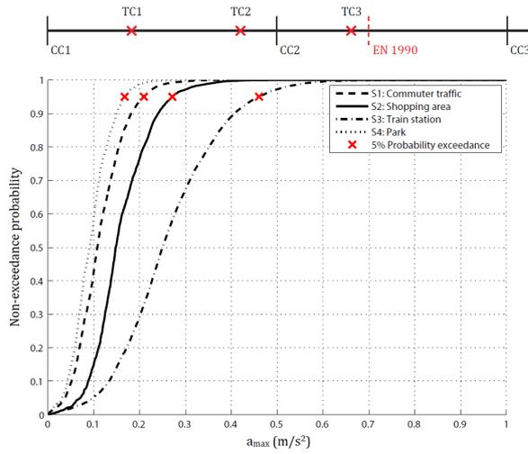
Figure 12.21: Cumulative density functions of the maximum expected accelerations per single pedestrian for the scenarios based on densities and L = 100 m
