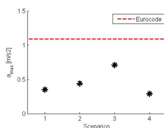
Figure 12.7: Results of the maximum accelerations for the four scenarios based on densities for L = 50m
