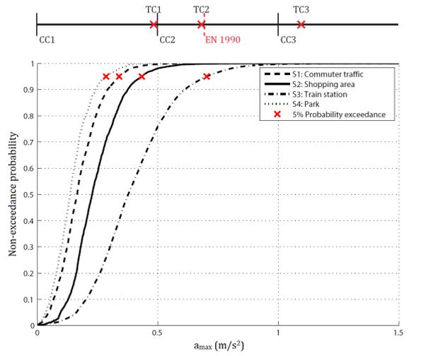
Figure 12.19: Cumulative density functions of the maximum expected accelerations per single pedestrian for the scenarios based on densities and  $L = 50 \text{ m}$
