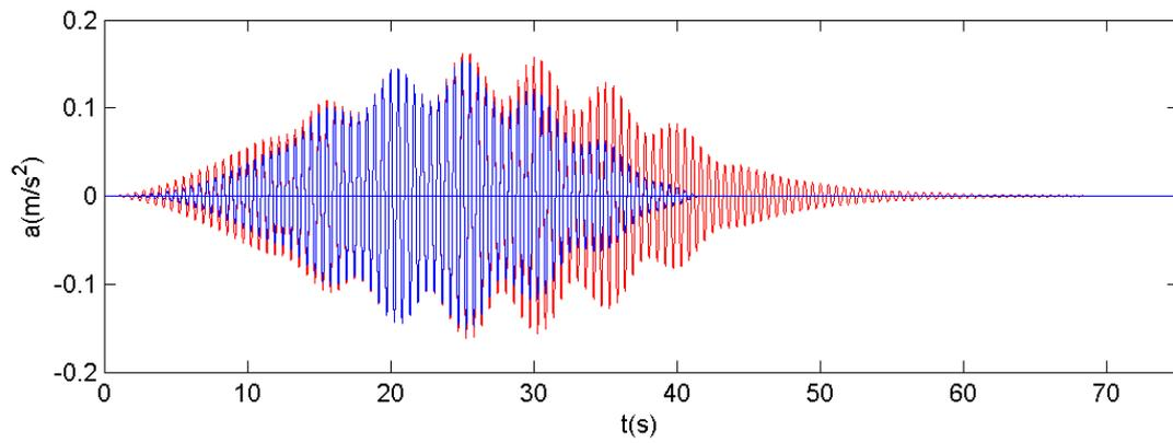
Figure D.11: Acceleration of the bridge (red) due to two separate pedestrians for the first mode at  $x = 25$  m and the accelerations the first pedestrian experiences (blue) when crossing the bridge - Matlab
