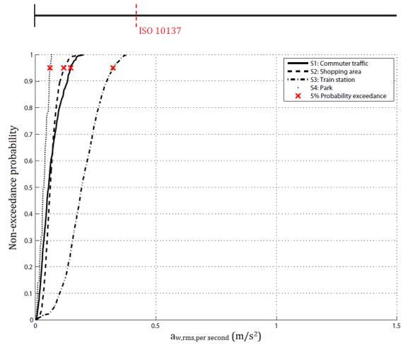
Figure 12.26: Cumulative density functions of the expected r.m.s. per second of the weighted accelerations per single pedestrian for the scenarios based on group formation and  $L = 50$  m
