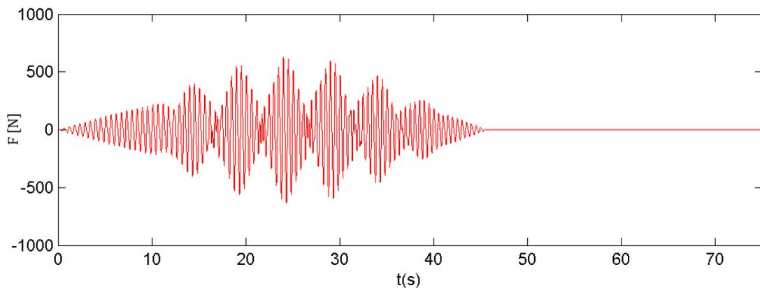
Figure D.9: Force of two combined pedestrians crossing the footbridge with  $L = 50$  m - Matlab
