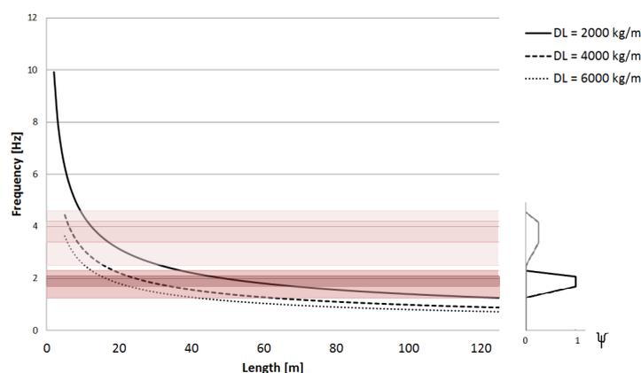
Figure 6.1: Relation between natural frequency and length of simply supported footbridges with different dead loads
