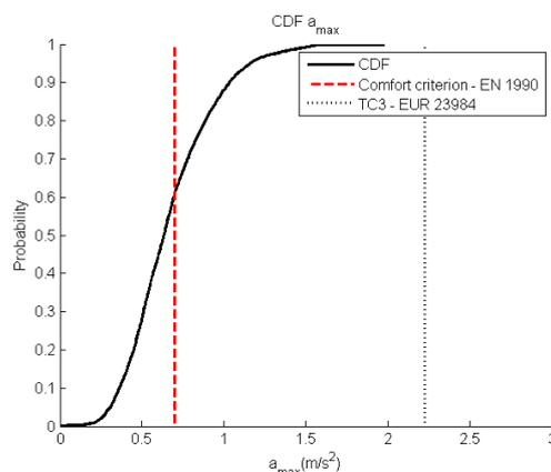
Figure F2: Cumulative density function of the maximum accelerations per single pedestrian crossing the bridge within a crowd density of  $0.5 P/m^2$ , compared with the maximum acceleration calculated with EUR 23984 for the bridge  $L = 12$  m
