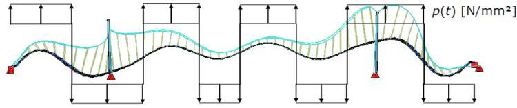
Figure C.1: Application of a harmonic load according to mode shape  $\phi(x)$  [6]
