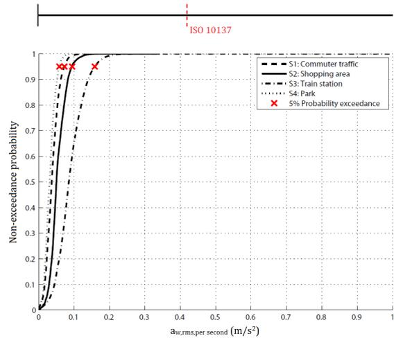
Figure 12.22: Cumulative density functions of the expected r.m.s. per second of the weighted accelerations per single pedestrian for the scenarios based on densities and L = 100 m
