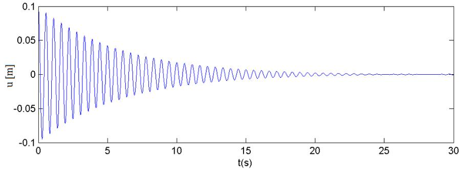
Figure D.1: Response of the structure with only an initial excitation - Matlab model
