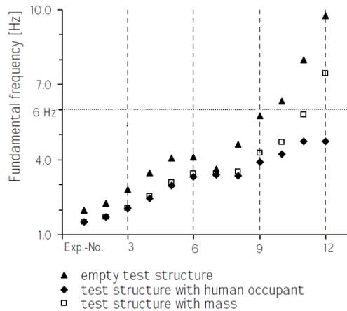
Figure 5.13: The influence of a standing human occupant and an equivalent mass on fundamental natural frequencies [50]
