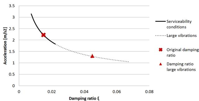
Figure 6.27: Deviation in damping ratio for a simply supported bridge  $L = 10$  m
