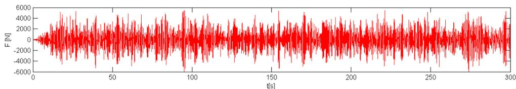
Figure 11.27: Example of the pedestrian loading for a crowd with a density of  $0.5 \text{ P/m}^2$  walking across a bridge with  $L = 50$  m
