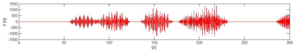
Figure 11.26: Typical pedestrian loading for several small groups walking across a bridge with  $L = 50$  m
