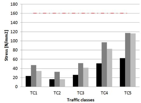
Figure 6.16: Stresses for a bridge L = 12m
