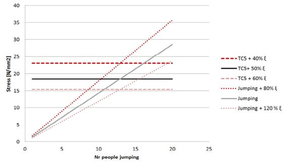
Figure 6.24: Stresses and acceleration for a bridge L = 100 m
