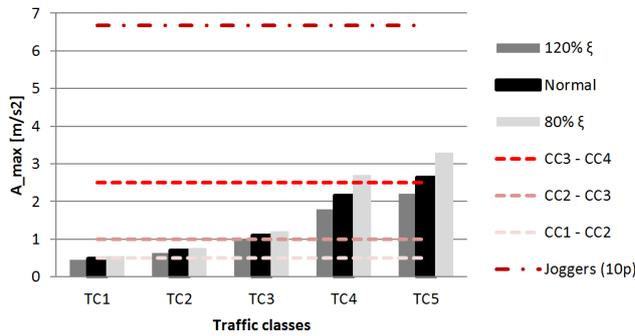
Figure 6.31: Accelerations for a bridge L = 50 m with different damping properties
