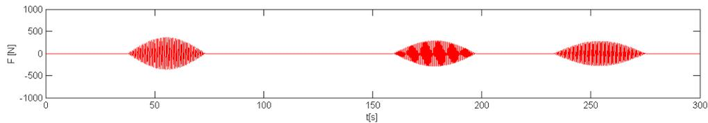
Figure 11.25: Typical pedestrian loading for three individual pedestrians walking across a bridge with  $L = 50$  m
