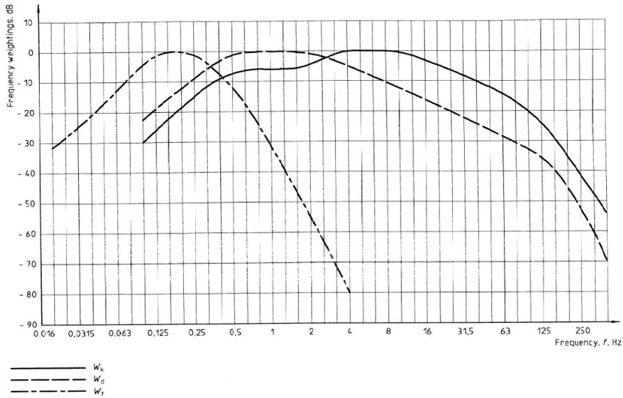
Figure E.2: Frequency weighting curves for principal weightings, with  $W_k$  as the frequency weighting curve that has to be applied in the case of comfort for standing persons [67]
