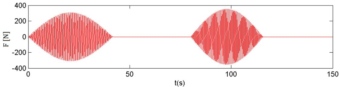
Figure D.5: Force of two separate pedestrians crossing the footbridge with  $L = 50$  m - Matlab
