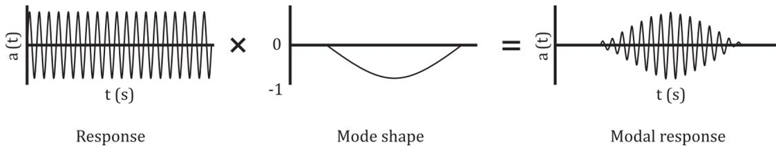
Figure 10.5: Result modal response: schematic representation of the accelerations a pedestrian experiences when crossing the bridge
