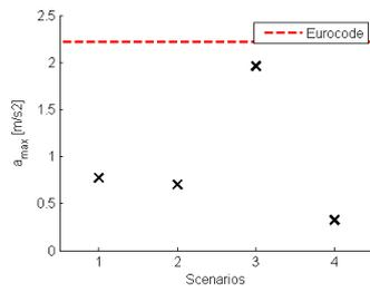
Figure 12.9: Results of the maximum accelerations for the four scenarios based on group formation for L = 12m
