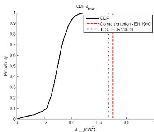
Figure E4: Cumulative density function of the maximum accelerations per single pedestrian crossing the bridge within a crowd density of  $0.5 P/m^2$ , compared with the maximum acceleration calculated with EUR 23984 for the bridge  $L = 100$  m
