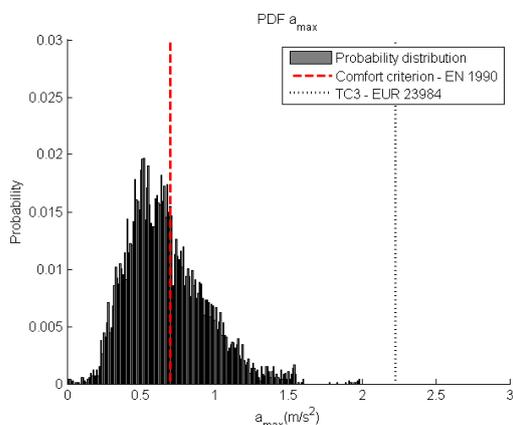
Figure F1: Probability distribution of the maximum accelerations per single pedestrian crossing the bridge within a crowd density of  $0.5 P/m^2$ , compared with the maximum acceleration calculated with EUR 23984 for the bridge  $L = 12$  m
