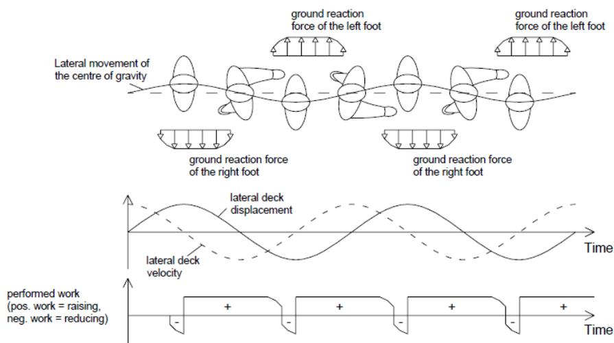
Figure 5.12: Schematic description of synchronous walking in lateral direction [23]
