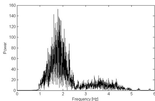
Figure 11.24: Walking frequencies of the pedestrians plotted in the frequency domain as used in the case study
