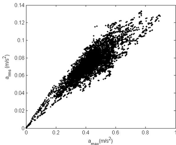
Figure 12.15: The correlation between the maximum acceleration and the r.m.s. of the acceleration per single pedestrian for a bridge  $L = 50$  m and a traffic density of  $0.5 P/m^2$
