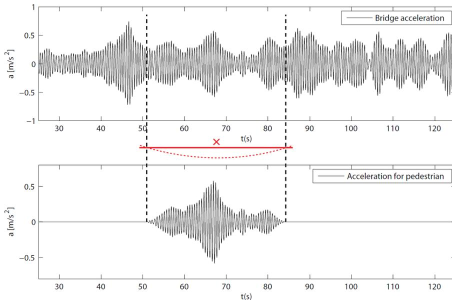
Figure 11.30: Top figure: accelerations of the bridge with  $L = 50 \text{ m}$  and a crowd loading of  $0.5 \text{ P/m}^2$ ; bottom figure: the accelerations a pedestrian experiences when crossing the bridge, for the first natural frequency
