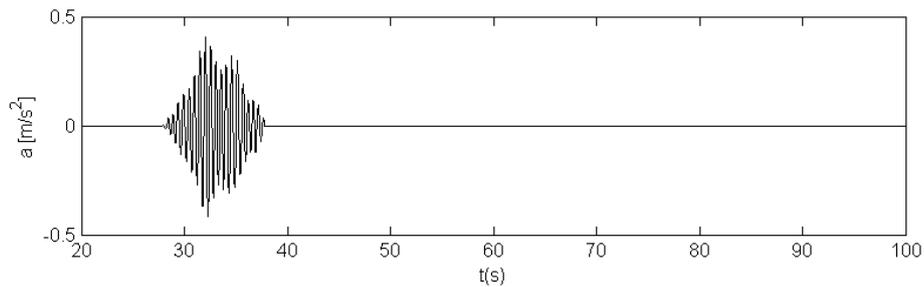
Figure 11.31: Example of a typical acceleration signal which a single individual pedestrian perceives crossing a footbridge with  $L = 12 \text{ m}$
