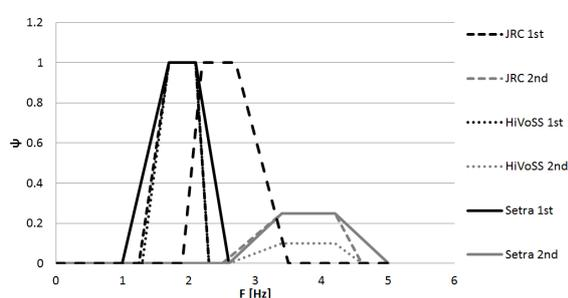
Figure 5.4: Reduction coefficient for the vertical and longitudinal direction according to several guidelines
