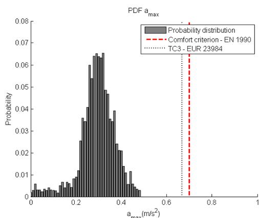
Figure E3: Probability distribution of the maximum accelerations per single pedestrian crossing the bridge within a crowd density of  $0.5 P/m^2$ , compared with the maximum acceleration calculated with EUR 23984 for the bridge  $L = 100$  m
