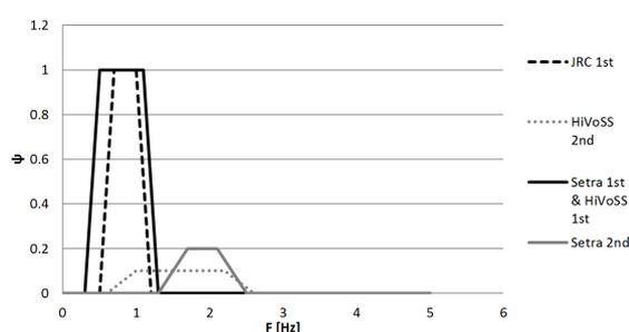
Figure 5.5: Reduction coefficient for the lateral direction according to several guidelines
