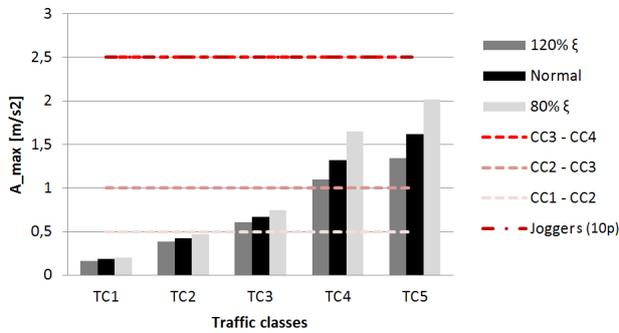
Figure 6.33: Accelerations for a bridge L = 100 m with different damping properties
