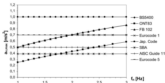
Figure 5.1: Limit values of vertical acceleration according to International Standards [14]
