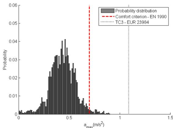
Figure 11.37: Probability distribution of the maximum accelerations per single pedestrian crossing the bridge within a crowd density of  $0.5 \text{ P/m}^2$ , compared with the maximum acceleration calculated with EUR 23984 for the bridge  $L = 50 \text{ m}$
