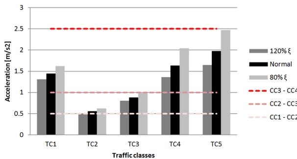
Figure 6.35: Accelerations in a cantilever beam footbridge of 2.5 m
