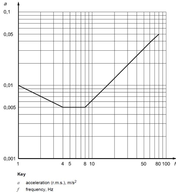
Figure 10.12: Base curve for acceleration in the vertical direction according to ISO 10137 [68]
