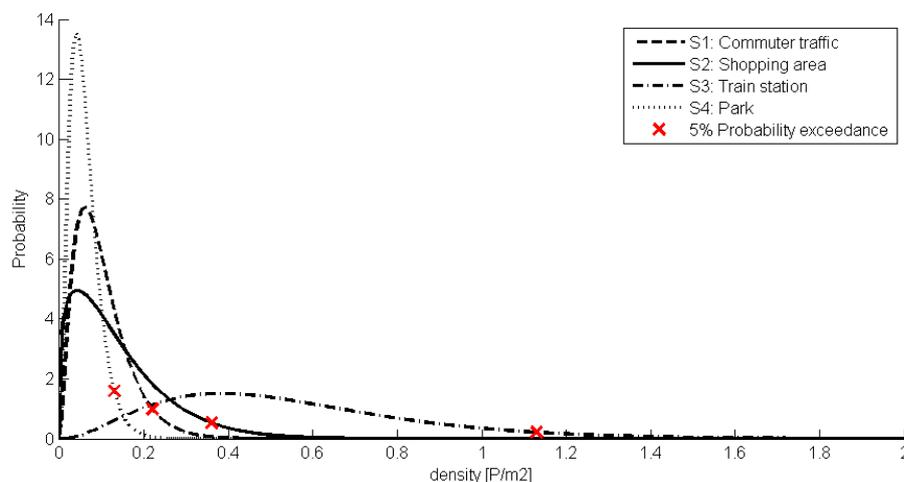
Figure 12.1: Probability density functions including the 5 percentage exceedance level per bridge for the four scenarios based on densities
