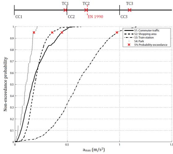
Figure 12.25: Cumulative density functions of the maximum expected accelerations per single pedestrian for the scenarios based on group formation and  $L = 50$  m
