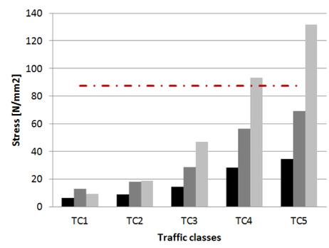
Figure 6.18: Stresses for a bridge L = 50m
