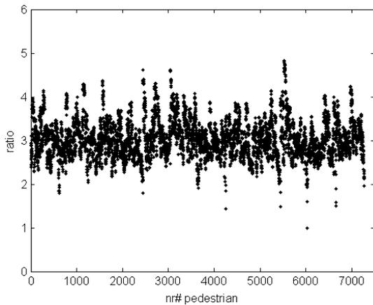
Figure 11.34: The crest factor per single pedestrian for a bridge L = 50 m for the total time
