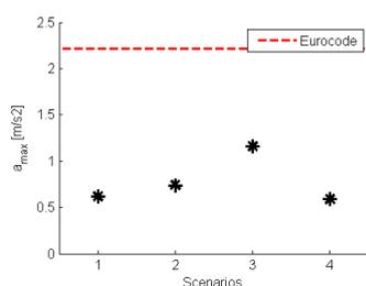
Figure 12.6: Results of the maximum accelerations for the four scenarios based on densities for L = 12m
