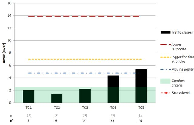
Figure 6.7: Accelerations for beam L = 12 m
