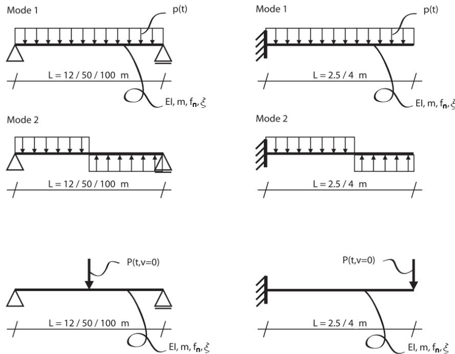
Figure 6.6: Load models for the first and second mode of the simply supported beam and for the cantilever beam
