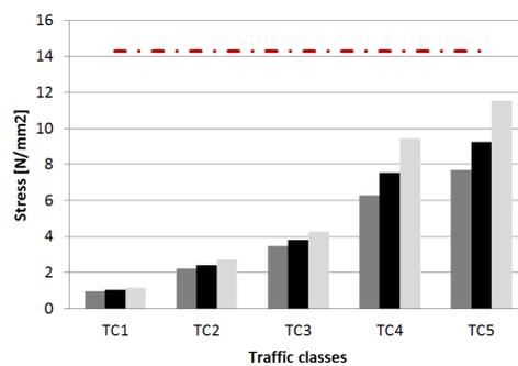
Figure 6.34: Stresses for a bridge L = 100 m with different damping properties
