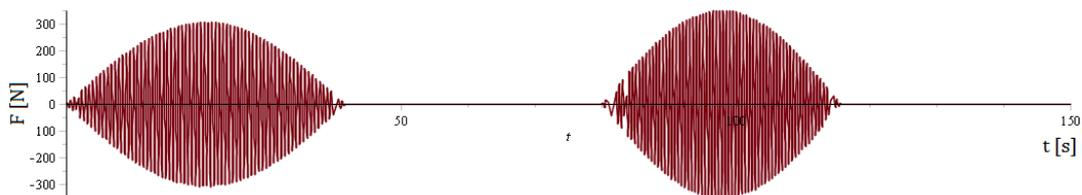
Figure D.6: Force of two separate pedestrians crossing the footbridge with  $L = 50$  m - Maple
