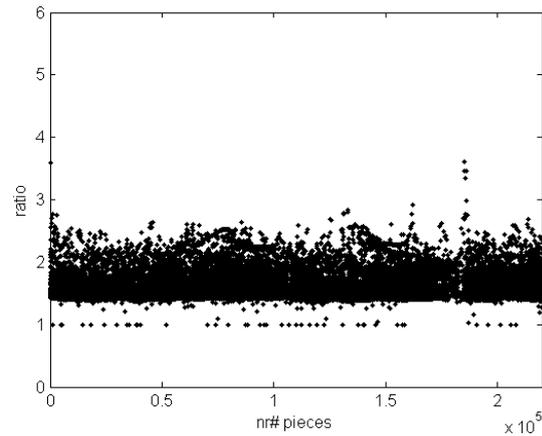
Figure 11.35: The crest factor per single pedestrian for a bridge L = 50 m per second
