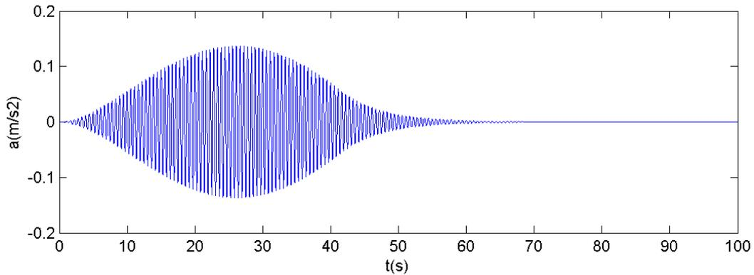
Figure D.3: Acceleration of the bridge due to a single pedestrian for the first mode at  $x = 25$  m - Matlab
