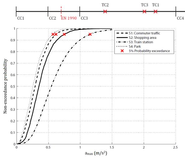
Figure 12.17: Cumulative density functions of the maximum expected accelerations per single pedestrian for the scenarios based on densities and  $L = 12 \text{ m}$
