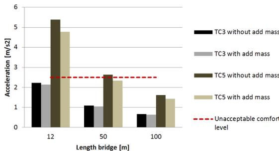
Figure 6.39: Change in acceleration by taking into account additional mass due to pedestrians
