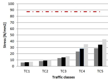
Figure 6.32: Stresses for a bridge L = 50 m with different damping properties
