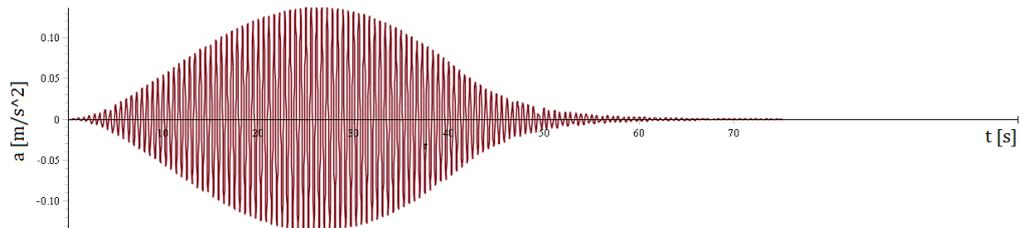
Figure D.4: Acceleration of the bridge due to a single pedestrian for the first mode at  $x = 25$  m - Maple
