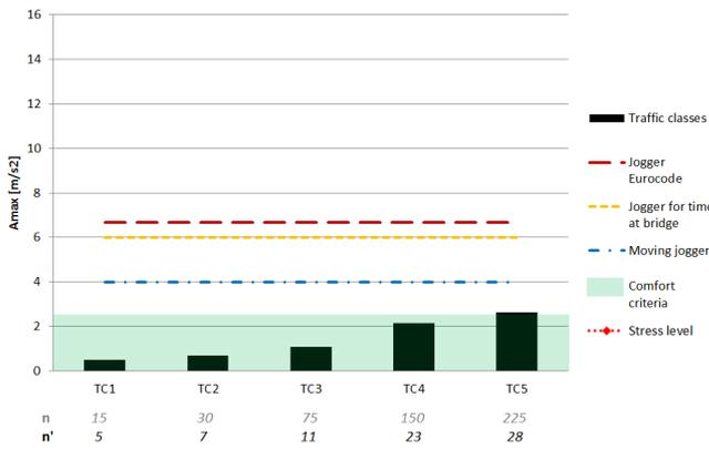
Figure 6.9: Accelerations for beam L = 50 m
