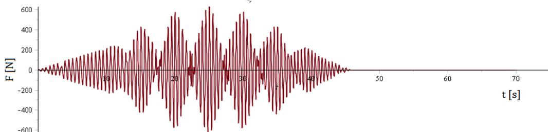
Figure D.10: Force of two combined pedestrians crossing the footbridge with  $L = 50$  m - Maple
