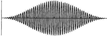
Figure 10.8: Transient oscillatory motion: general acceleration signal a single pedestrian is exposed to when crossing a bridge [66]
