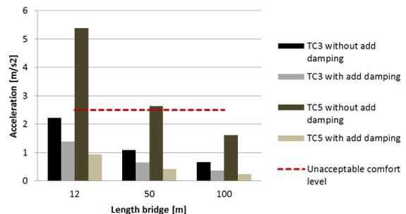
Figure 6.40: Change in acceleration by taking into account additional damping due to pedestrians
