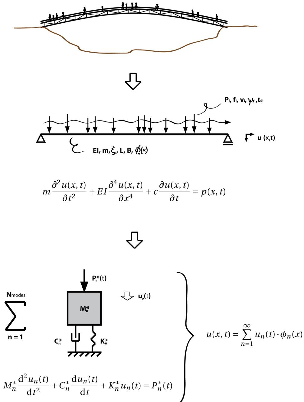
Figure 10.4: Overview of the steps taken for modelling pedestrians crossing a footbridge in Matlab
