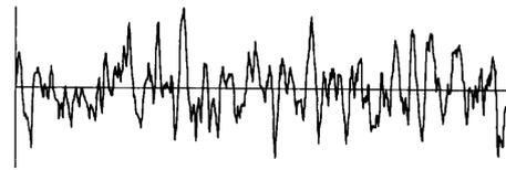
Figure 10.9: Random oscillatory motion: general acceleration signal a flow pedestrians is exposed to when crossing a bridge [66]
