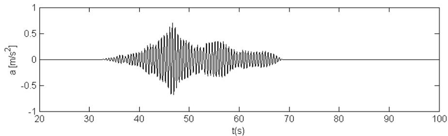
Figure 11.32: Example of a typical acceleration signal which a single individual pedestrian perceives crossing a footbridge with  $L = 50 \text{ m}$
