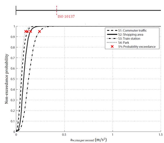
Figure 12.20: Cumulative density functions of the expected r.m.s. per second of the weighted accelerations per single pedestrian for the scenarios based on densities and  $L = 50 \text{ m}$
