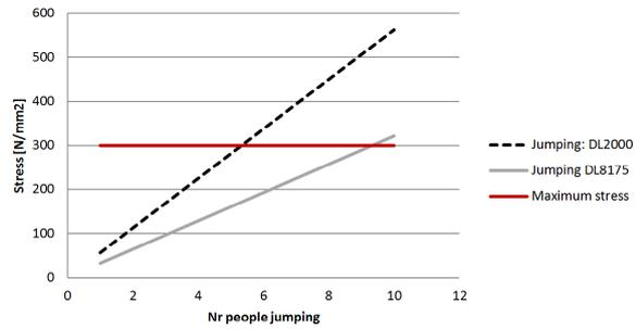
Figure 6.22: Stresses for a bridge L = 12 m with low dead load of 2000 [N/m<sup>2</sup>]
