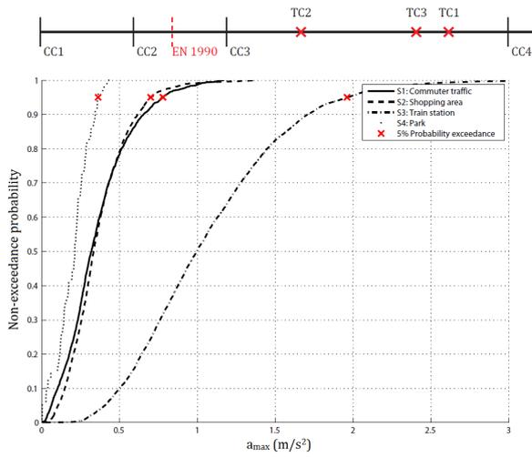
Figure 12.23: Cumulative density functions of the maximum expected accelerations per single pedestrian for the scenarios based on group formation and L = 12 m
