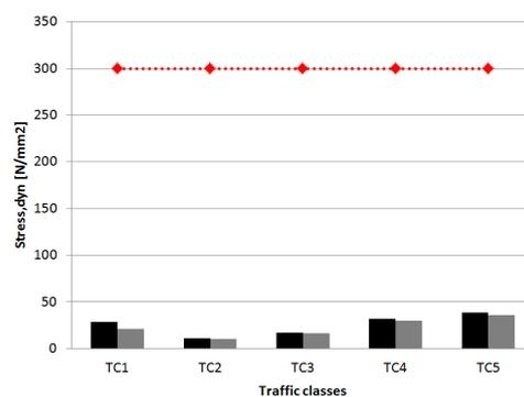
Figure 6.14: Stresses for different traffic classes in case of a cantilever footbridge
