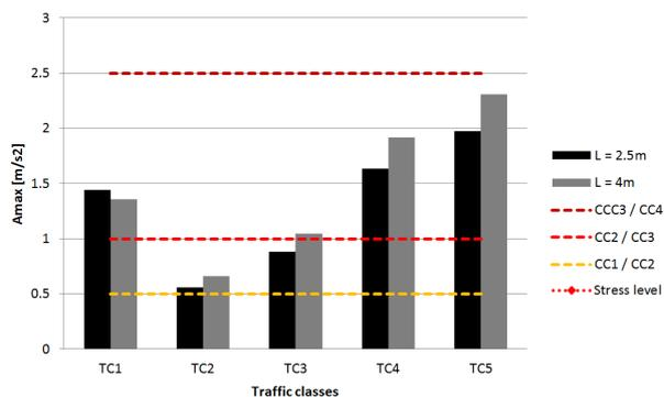
Figure 6.13: Acceleration for different traffic classes in case of a cantilever footbridge
