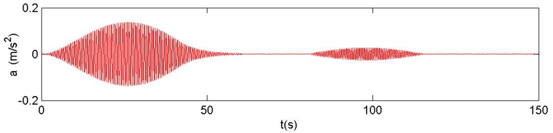
Figure D.7: Acceleration of the bridge due to two separate pedestrians for the first mode at  $x = 25$  m - Matlab
