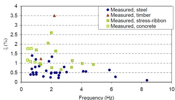
Figure 5.10: Measured damping ratios under service loads: variation with natural frequency [6]
