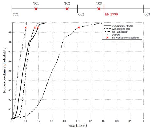
Figure 12.27: Cumulative density functions of the maximum expected accelerations per single pedestrian for the scenarios based on group formation and  $L = 100$  m
