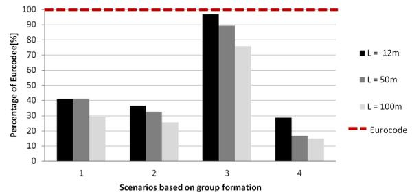
Figure 12.13: Comparison of the results of the accelerations for the scenarios based on group formation with the expected bridge acceleration of the Eurocode - expressed in percentage [%] of the Eurocode acceleration
