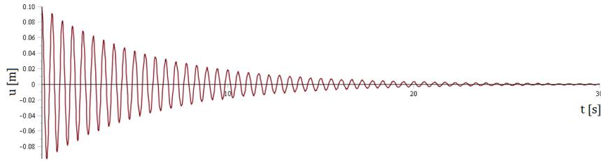
Figure D.2: Response of the structure with only an initial excitation - analytical solution plotted with Maple
