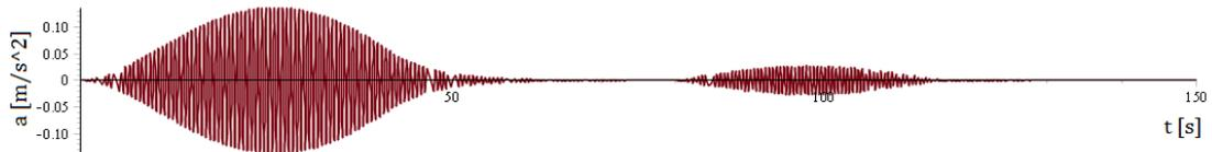
Figure D.8: Acceleration of the bridge due to two separate pedestrians for the first mode at  $x = 25$  m - Maple
