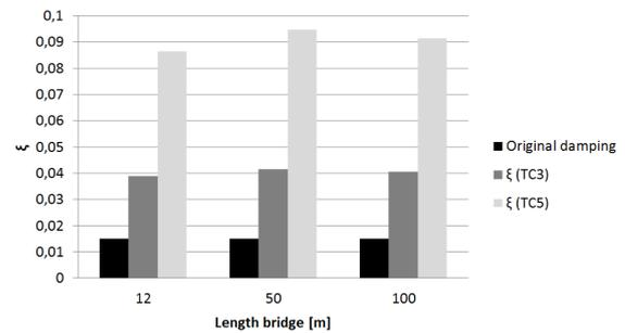
Figure 6.38: Change in damping by taking into account additional damping due to pedestrians
