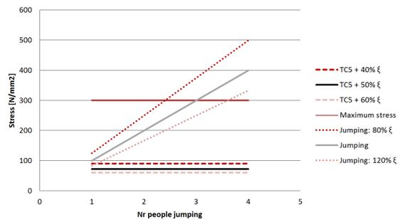
Figure 6.26: Stresses in a cantilever beam footbridge of 4 m
