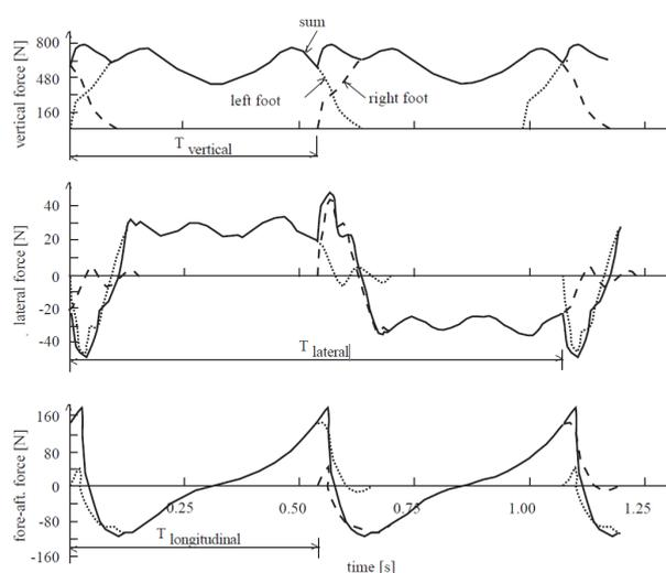
Figure 3.1: Typical shapes of walking force in vertical, lateral and longitudinal directions [10]
