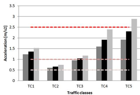
Figure 6.36: Accelerations in a cantilever beam footbridge of 4 m
