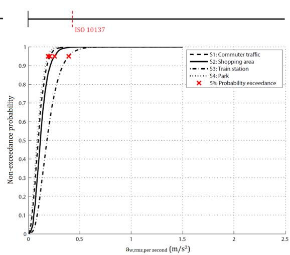
Figure 12.18: Cumulative density functions of the expected r.m.s. per second of the weighted accelerations per single pedestrian for the scenarios based on densities and  $L = 12 \text{ m}$
