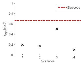
Figure 12.11: Results of the maximum accelerations for the four scenarios based on group formation for L = 100m
