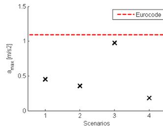
Figure 12.10: Results of the maximum accelerations for the four scenarios based on group formation for L = 50m
