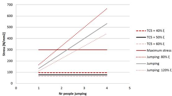
Figure 6.25: Stresses in a cantilever beam footbridge of 2.5 m
