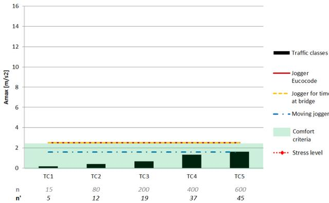
Figure 6.11: Accelerations for beam L = 100 m
