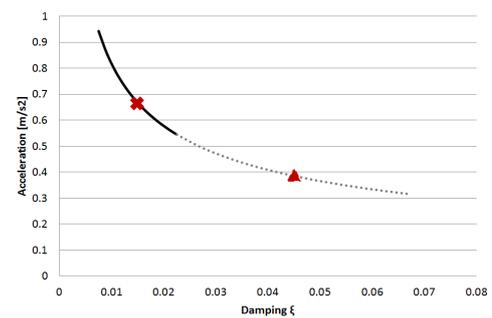
Figure 6.28: Deviation in damping ratio for a simply supported bridge  $L = 100$  m
