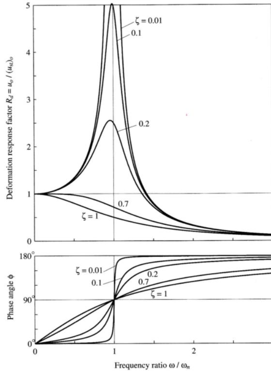
Figure 3.7: Deformation response factor for a damped system excited by a harmonic force [19]
