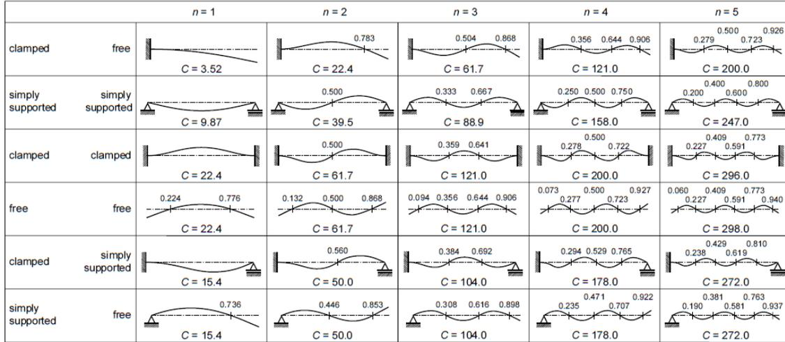
Figure 3.6: Natural frequencies and eigenmodes of beams with constant  $EI\rho A$
