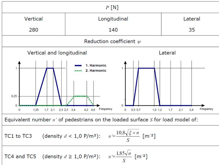
Figure 4.7: Parameters for the harmonic load model [6]
