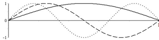
Figure 6.3: First three mode shapes for a simply supported beams
