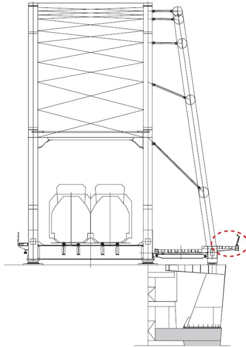
Figure 6.5: Example of a cantilever footbridge at the "Snelbinder" in Nijmegen in the red dotted circle [55]
