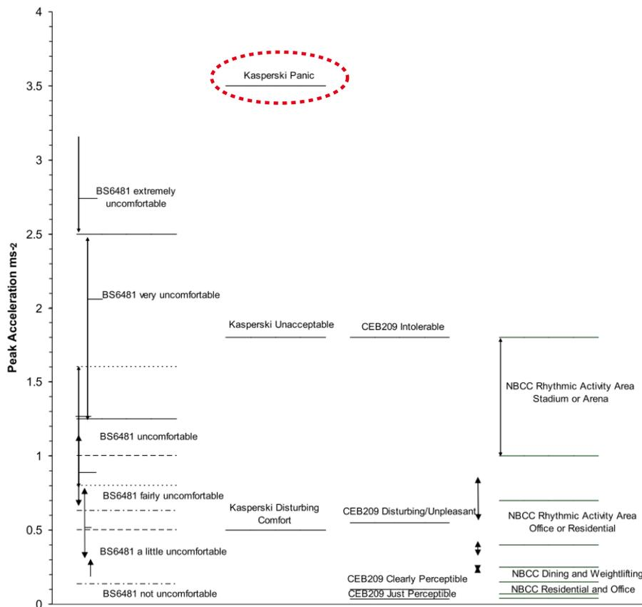
Figure 10.1: Summary of acceleration limit serviceability criteria for grandstands by Browning with the panic limit level of accelerations according to Kasperski in the red circle [61]
