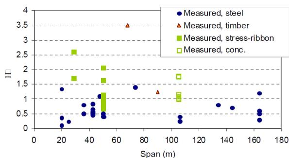
Figure 5.11: Measured damping ratios under service loads: variation with span [6]
