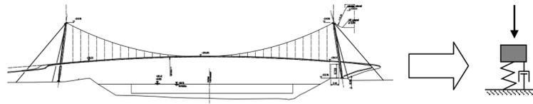
Figure 4.9: Equivalent SDOF oscillator for one natural frequency [6]
