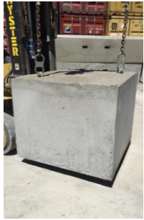
Figure 63: Lifting concrete block with built-in hooks [274]
