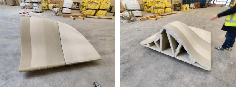
Figure 38: The Perfect Wave smooth outside (left) and internal structure (right)
