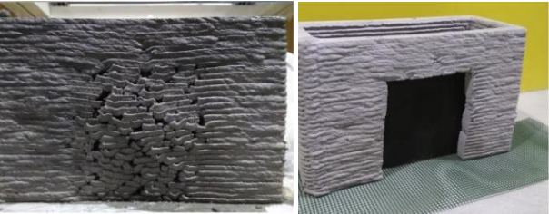
Figure 42: Printed supports (left) and resulting structure (right) [224]
