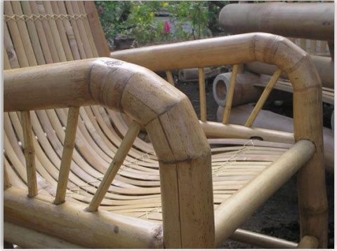
Figure 83: Bended bamboo through heat bending process [288]
