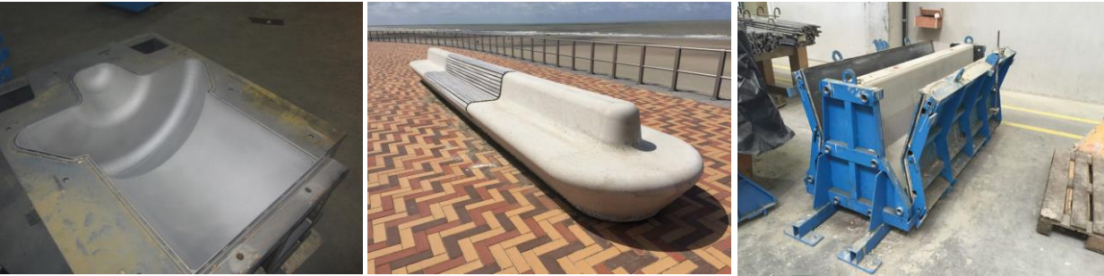
Figure 100: Mould to create structures with a sham edge [354]
