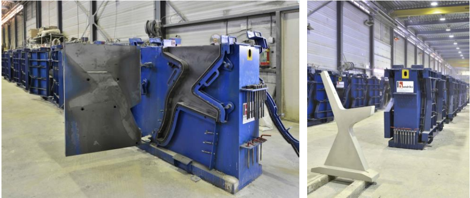
Figure 101: Mould to create flat structures (left) and final product (right) [355]
