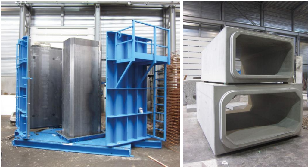
Figure 98: Mould to create tubular elements (left) and final product (right) [352]
