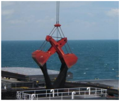
Figure 23: Scissor grab handling
