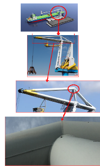
Figure 1. Fatigue critical tubular connection on upperarm of lemniscate crane
