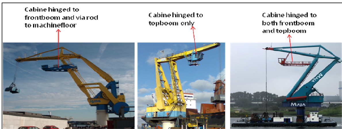
Figure 12: Cabin structure designs ( McDermoth, 2005)
