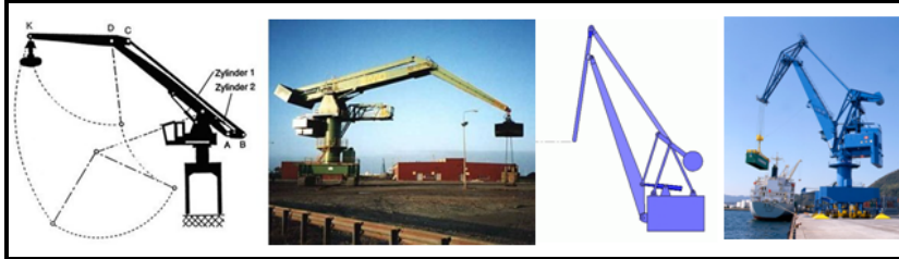
Figure 8: Applications of the four-bar linkage mechanism (Kaenders, 2007)
