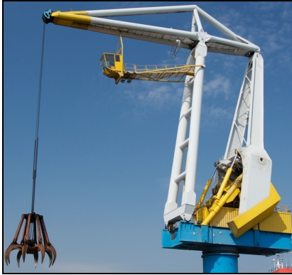
Figure 3: Study case-Cornelis Tromp 25t floating lemniscate crane (Maja Stuwadoors BV, 2016)
