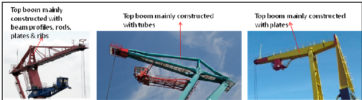
Figure 11: Upper arm structure designs ( McDermoth, 2005)
