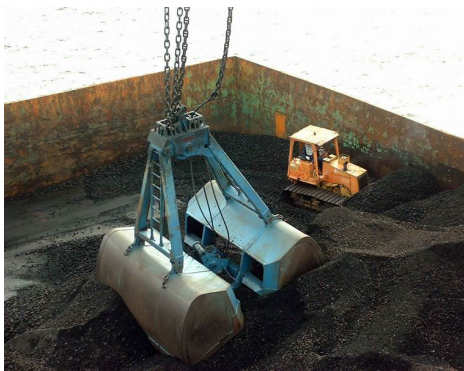
Figure 22: Clamshell grab handling
