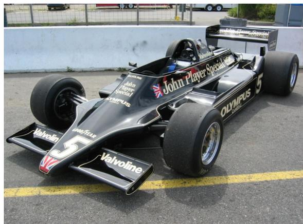
**Figure 1-1:** Lotus 79: First car to take full advantage of ground effects aerodynamics [1]
