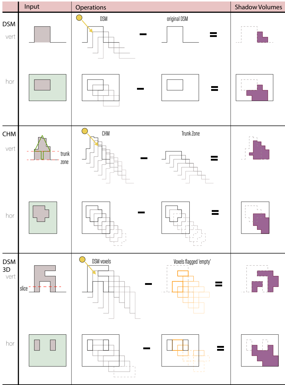
Figure 8: Explanation of the current methods of shadow casting for DSM and CHM, and the proposed method for 3D DSM shadow casting.
