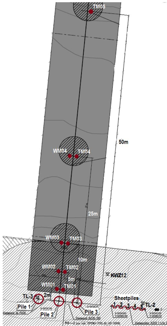
(a) Top view of pile installation test in the submerged slope, with the location of piles 1-3, sheet piles 1-5, sensors and CPTs KWZ12, TL-3 and TL-2.
