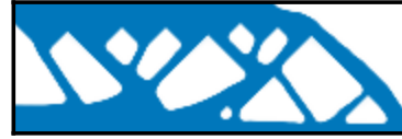
Figure 4.8: Reference single-material design for the MBB beam with \alpha^{(2)} = 45^\circ . Material properties according to Table 4.1.
