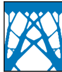
Figure 4.10: Reference single-material design for the MBB beam. Material properties according to Table 4.1.
