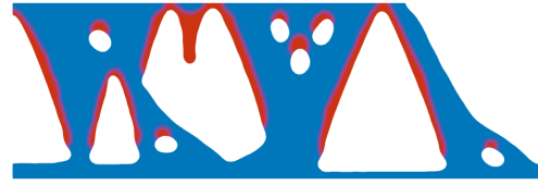
Figure 3.2: Example of a design with lenient critical temperatures for both materials. T_{cr}^{(1)} = 0.95 , and T_{cr}^{(2)} = 0.90 .
