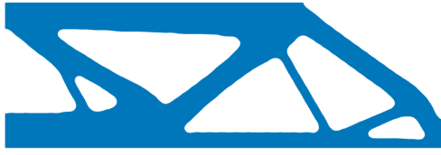
Figure 3.1: Reference multi-material design without a hotspot constraint. Note: Due to the nature of the compliance objective, the optimizer will always converge to a design made up of exclusively the material with the highest stiffness. c/c_{ref} = 254.9\%
