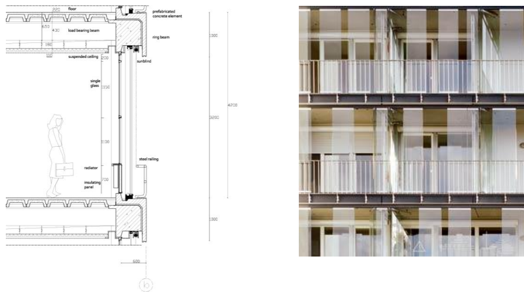
Figure 3.21: Concept detail wind and water proofing
