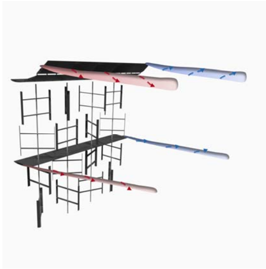
Figure 3. Render of the Multi-Rotor System (MRS) (right) velocity fields behind ABL-controlled setups illustrating the wing configuration. This image also with 2 wings, displaying u_x -velocity colored fields at provides a visual representation of the trailing vortices x/D = 1 . Setup with C_T = 0.72 and C_W = 0.88 generated by the wing tips, which will drive the vertical (vertical loading), featuring two blades. Full work in flux at both the wind farm scale and within the [Martins et al., 2024] Atmospheric Boundary Layer. Further details are available in [Broertjes et al., 2024].
