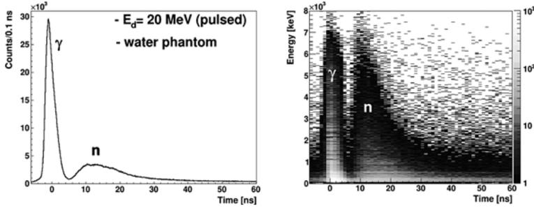
Figure 3: Time spectrum acquired with the LaBr<sub>3</sub>:Ce scintillator of the Compton camera from a pulsed deuteron beam ( $E_d = 20$  MeV) hitting a water phantom. Right panel: photon detection time (relative to RF trigger signal) vs. photon energy, left panel: projection on time axis.
