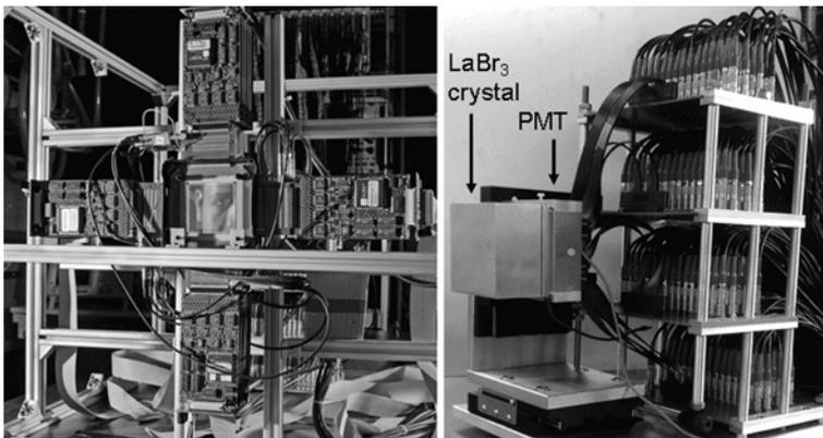
Figure 2: Left: Front of the Compton camera scatter/tracker array: double-sided Si-strip detector with ASIC-based signal processing electronics. Right: Absorbing  $\text{LaBr}_3\text{:Ce}$  scintillator.
