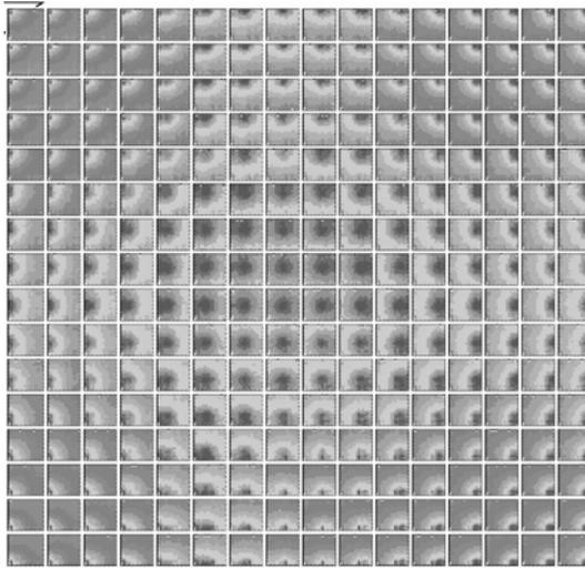
Figure 7: Grid scan of  $16 \times 16$  irradiation positions of the monolithic  $\text{LaBr}_3:\text{Ce}$  detector, using a 1 mm collimated  $^{137}\text{Cs}$  source and a grid step size of 3 mm in x and y direction. All 256 segments of the multi-anode PMT are individually read out. The resulting 2D ( $16 \times 16$ ) light amplitude distribution of each irradiation position clearly indicates the source position movement from the upper left corner to the lower right corner.
