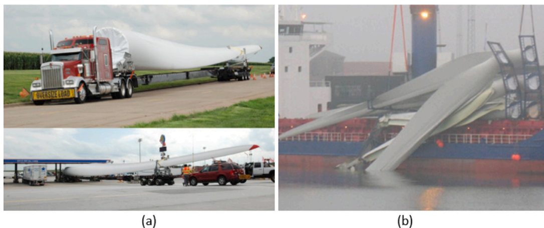
Fig. 6. (a) Onshore transportation of blade (permission taken from Elsevier [48]) (b) Blade damage during offshore transportation (permission taken from Skuld [49]).
