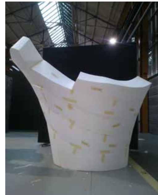
Leuven Pavillion. Technique: Robotically cut EPS modules.
