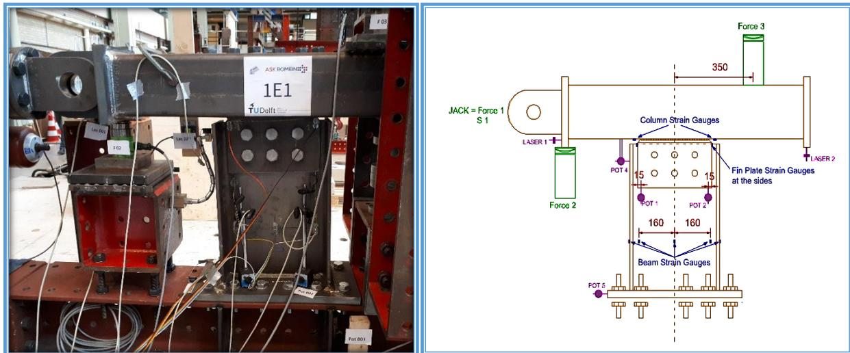
Figure 3 - 23: Instrumentation Location
