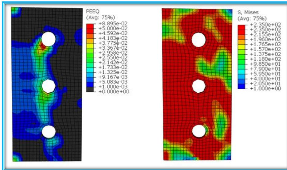
Figure 5- 6: Simple Joint - Strain/Stress Distribution of the Fin Plate (ABAQUS)
