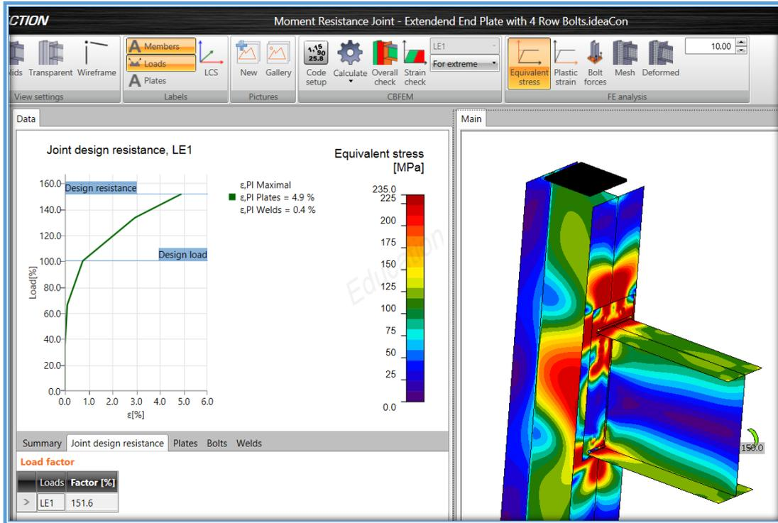
Figure A - 19: Joint Capacity Design
