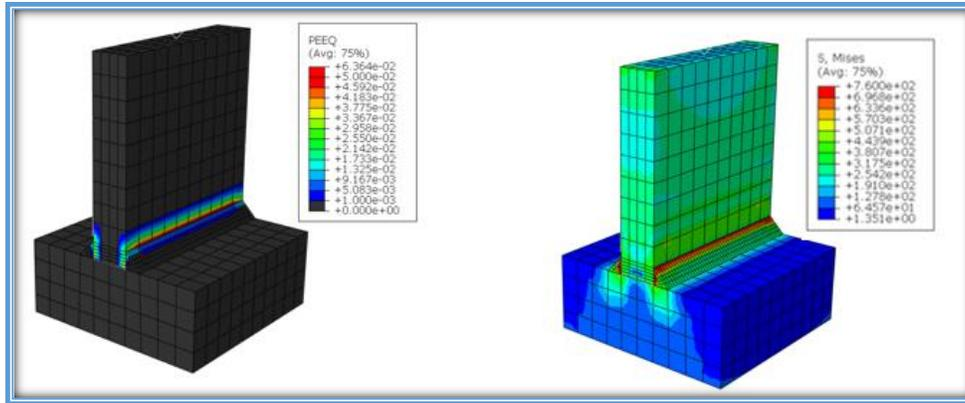
Figure 4 - 10: Strain/Stress Distribution in the Tension Analysis
