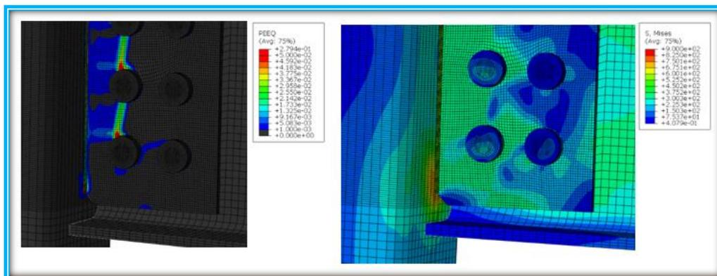
Figure 3 - 26: Experiment Joint - Strain/Stress Distribution (ABAQUS)
