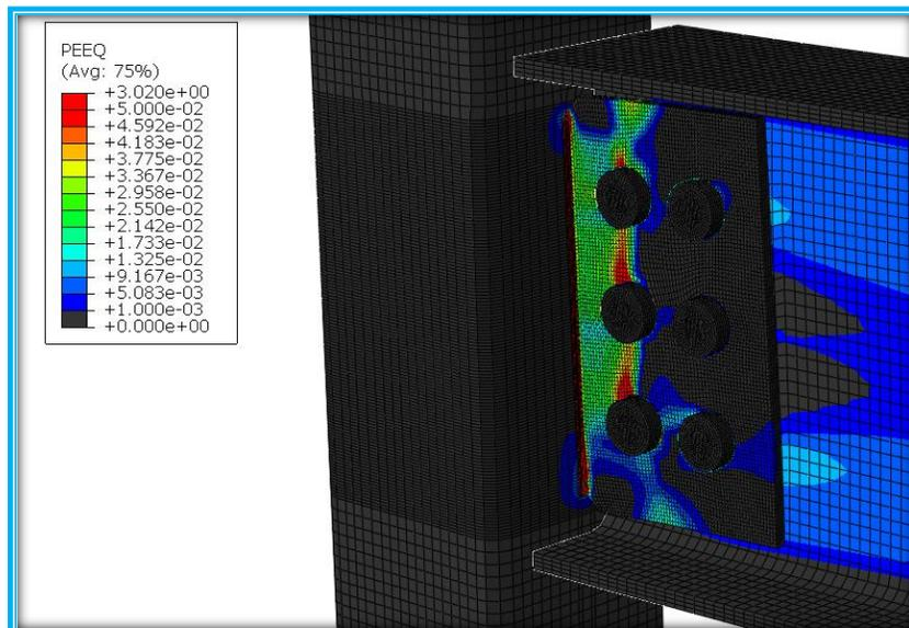
Figure 3 - 28: Experiment Joint - Plastic Strain Distribution (Nominal Hardening)
