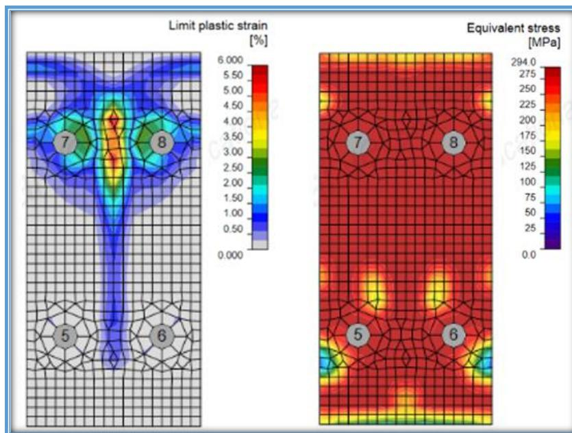
Figure 5- 13: Plastic Strain Distribution in the End Plate (IDEA StatiCa)
