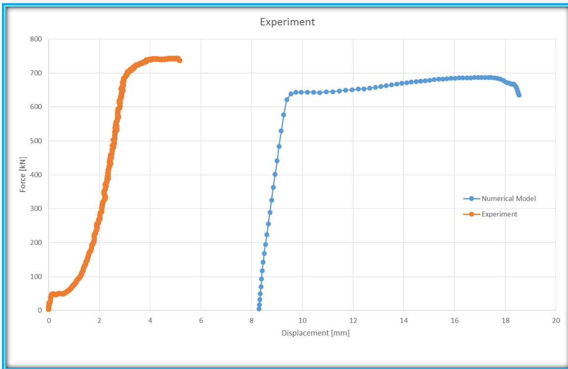
Figure 3 - 32: Numerical and Experiment Behavior of the Last Load Cycle
