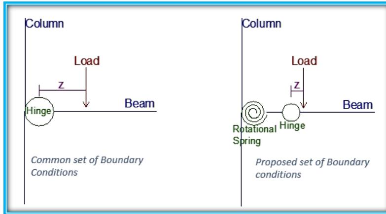
Figure 3 - 8: Common Boundary Conditions vs Proposed Boundary Conditions
