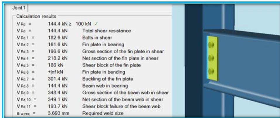
Figure 5- 3: Simple Joint - COP Results
