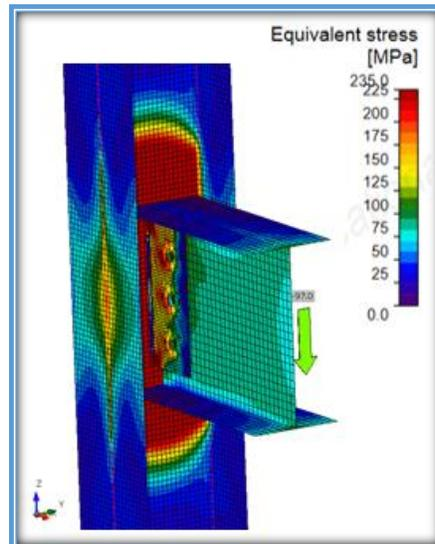
Figure 5- 5: Simple Joint - Stress Distribution (IDEA StatiCa)
