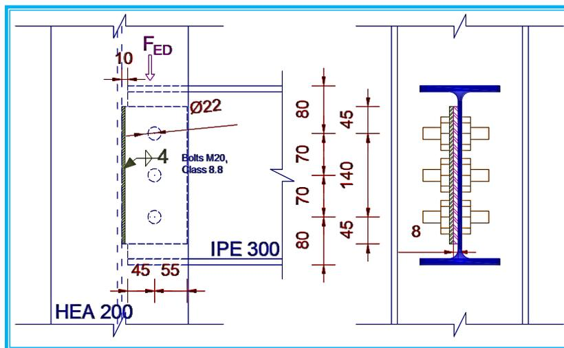
Figure 5- 1: Simple Joint - Geometry Detail
