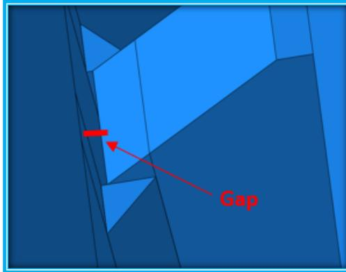
Figure 3 - 10: Gap between Column Face and Fin Plate
