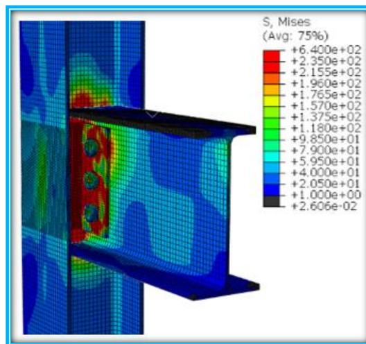
Figure 5- 7: Simple Joint - Stress Distribution (ABAQUS Ideal Plastic Material Model)
