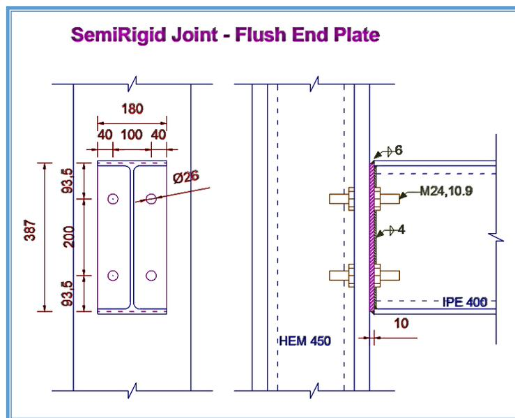
Figure 5- 11: Semi-Rigid Joint Details
