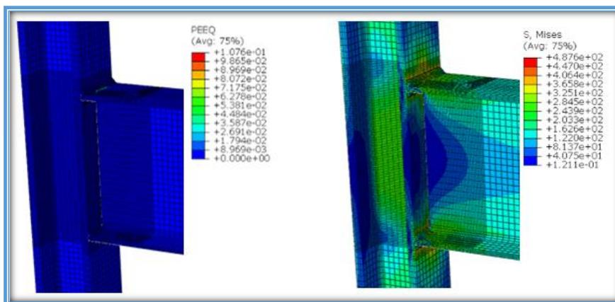
Figure 5- 24: Rigid Joint – Strain/Stress Distribution (ABAQUS - Ideal Plastic)
