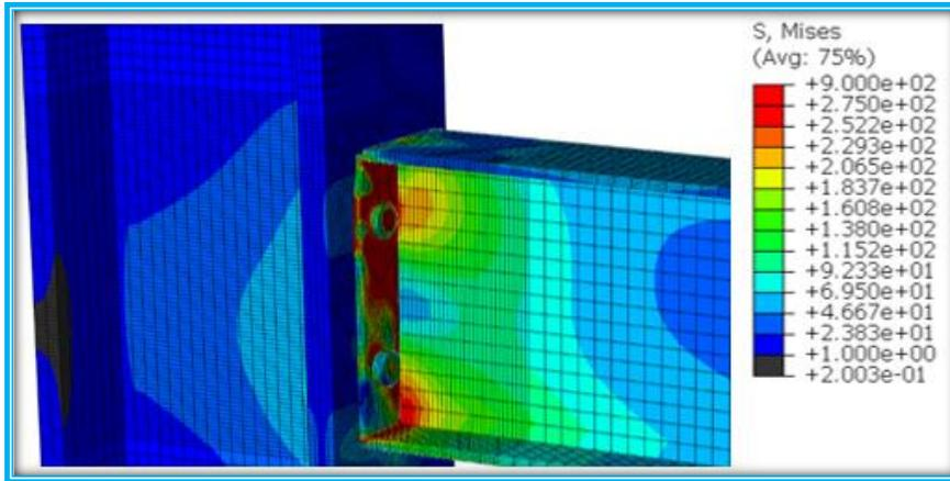
Figure 5- 16: Semi-Rigid Joint - Stress Distribution (ABAQUS - Ideal Plastic Model)
