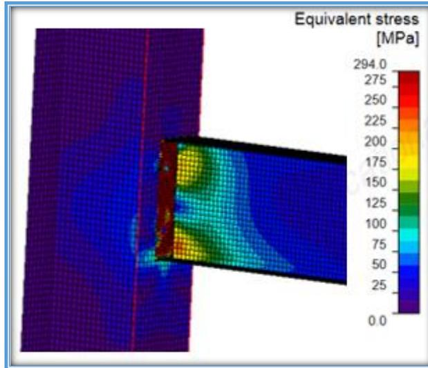
Figure 5- 14: Stress Distribution at the 5% Plastic Strain Limit
