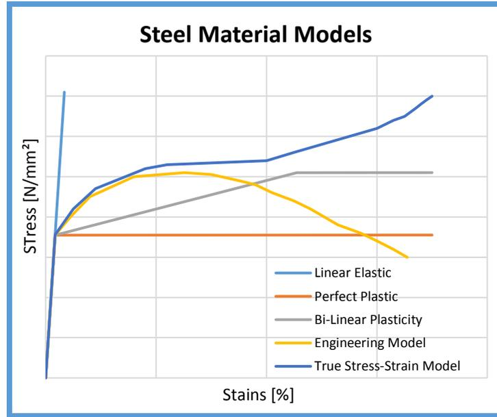
Figure A - 3: Steel Material Models
