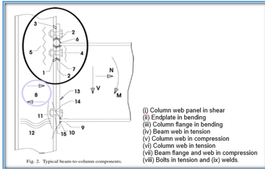
Figure 2 - 1: Typical Components from a Column-Beam Joint (Simões da Silva, 2008)
