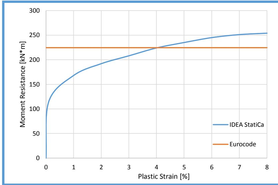
Figure A - 12: Moment vs Plastic Strain Curve
