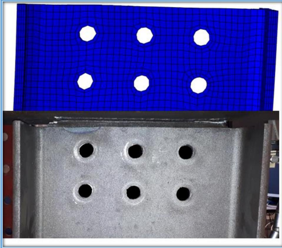
*Figure 3 - 41: Hole Deformation Pattern*
