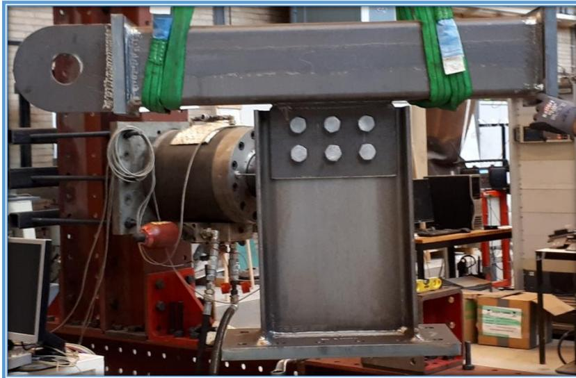
*Figure 1- 1: Experiment Specimen (Steel Joint)*
