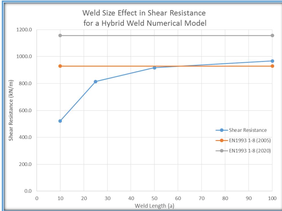
Figure 4 - 13: Results Comparison for the Shear Loaded Weld
