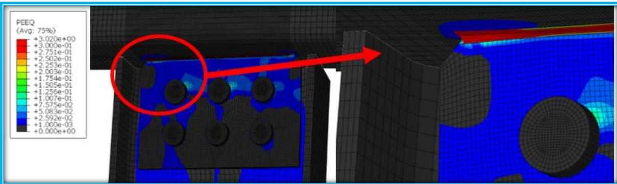
Figure 3 - 40: Plastic Strain at Ultimate Load
