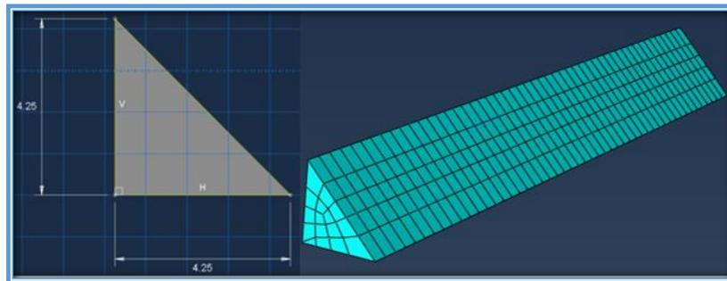
Figure 4 - 9: Weld Model – Throat thickness 3mm (ABAQUS)
