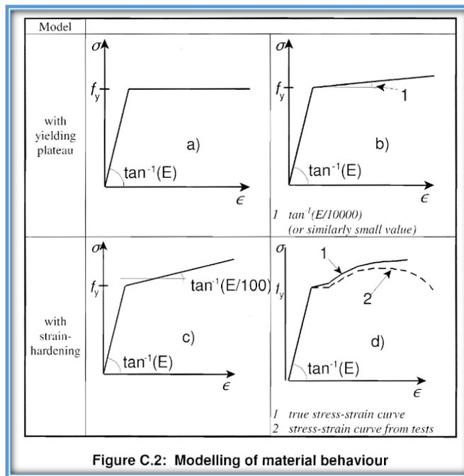
Figure 3 - 11: Material Models (EN1933 1-5 Annex C)
