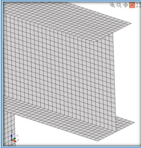
Figure A - 4: Finite Element Model of an "I" shape beam
