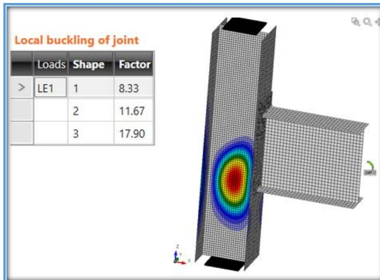
Figure A - 17: Buckling Analysis
