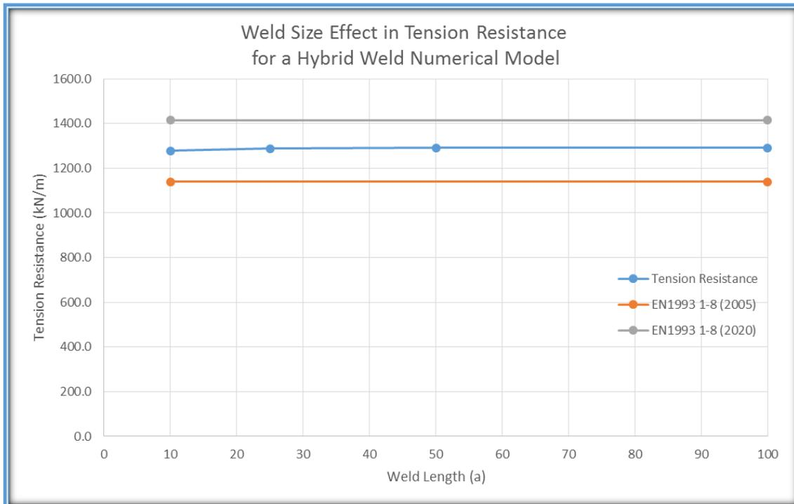
Figure 4 - 11: Results Comparison for the Tension Loaded Weld
