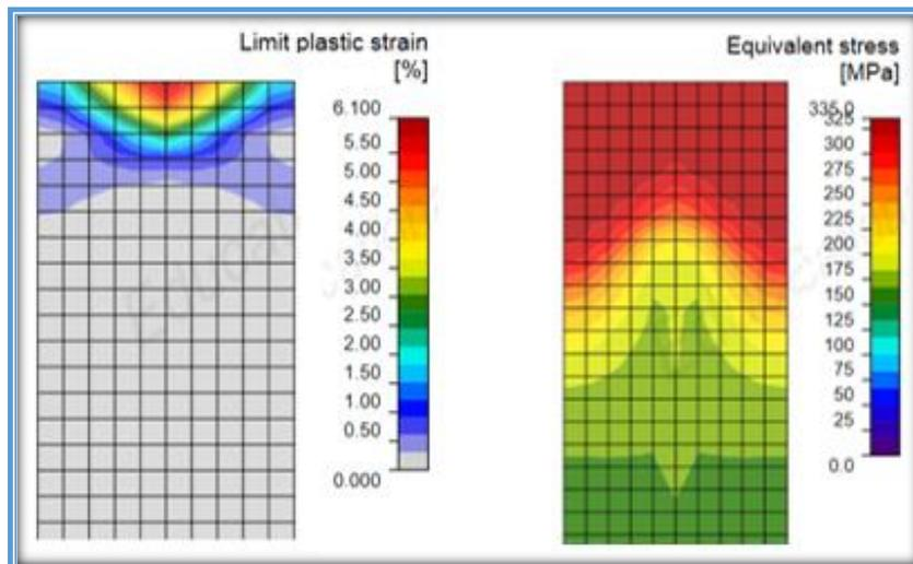
Figure 5- 21: Rigid Joint - Stress/Strain Distribution (IDEA StatiCa)
