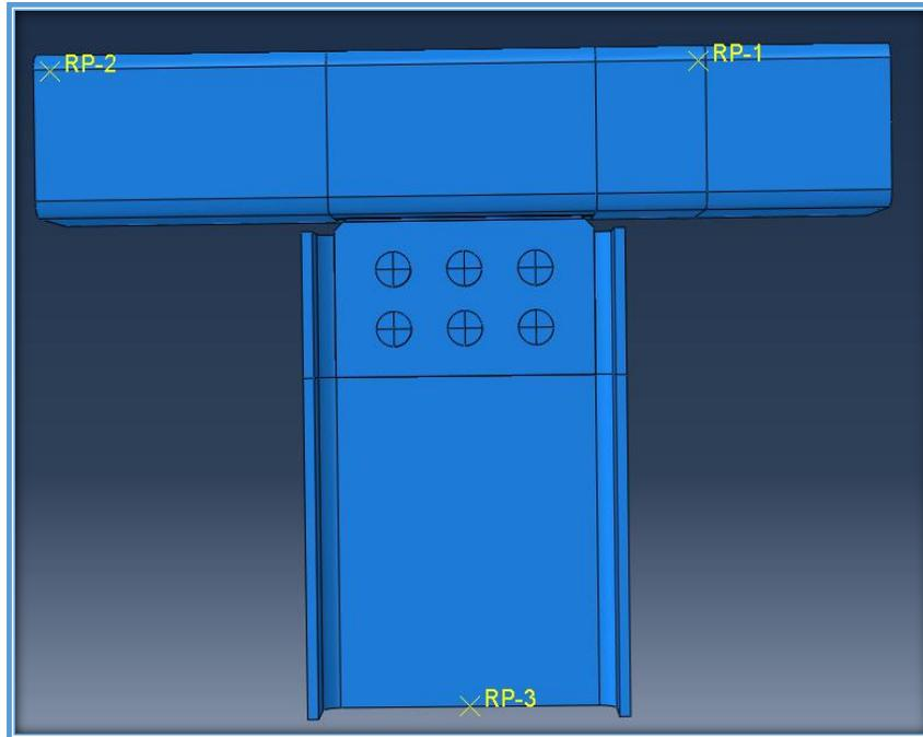
Figure 3 - 9: Location of the Master Nodes at the 3D Model
