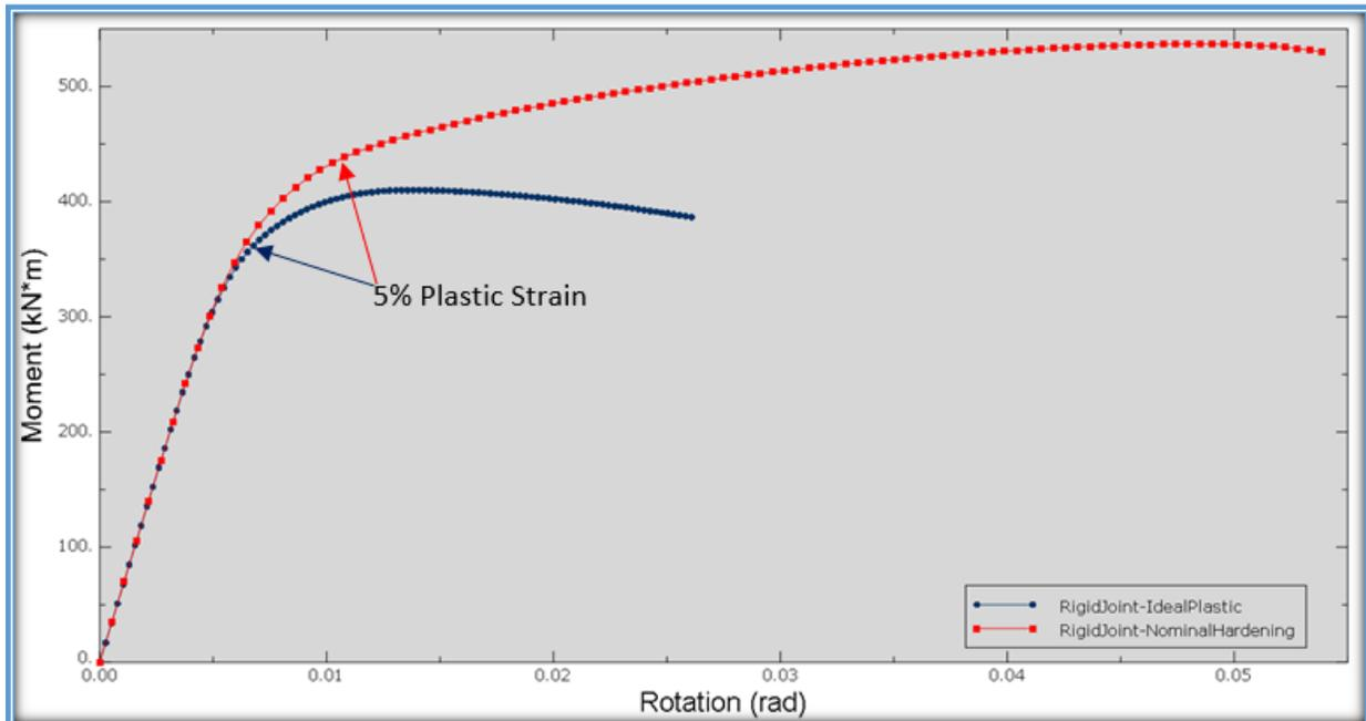
Figure 5- 25: Rigid Joint – Moment vs Rotation Curves (ABAQUS)
