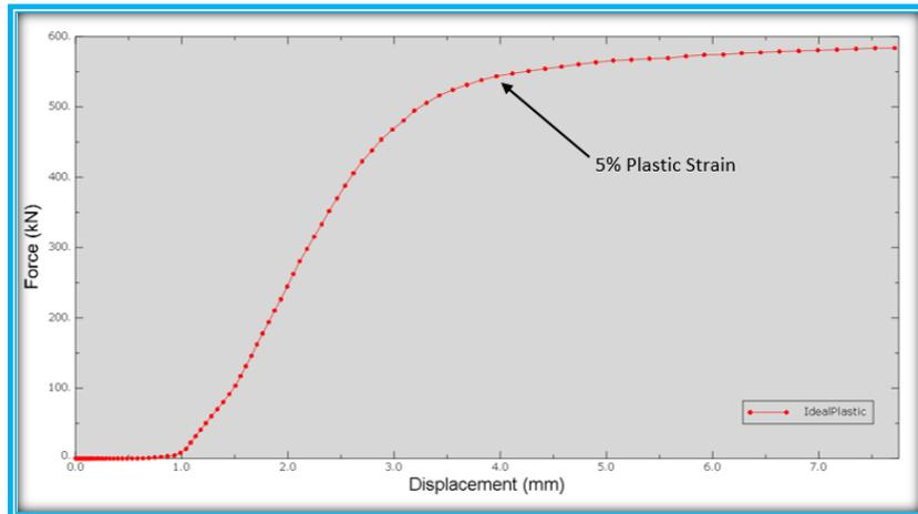
Figure 3 - 27: Experiment Joint - Force vs Displacement Curve (ABAQUS)
