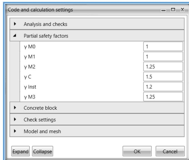
Figure A - 9: Partial Safety Factors Parameters
