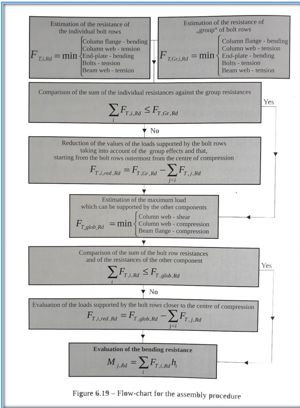
Figure 6.19 – Flow-chart for the assembly procedure
