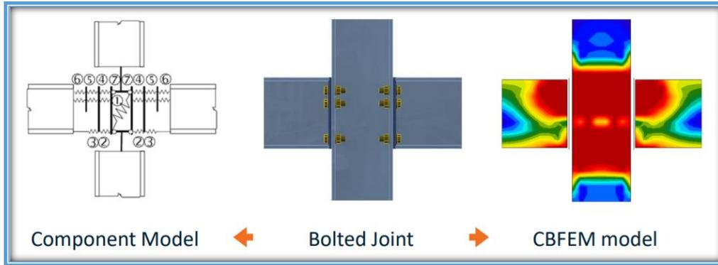
Figure A - 2: Component Model vs CBFEM Model
