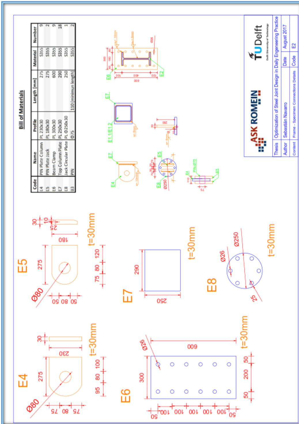
Figure 3 - 22: Workshop Drawings for the Connections to the Frame
