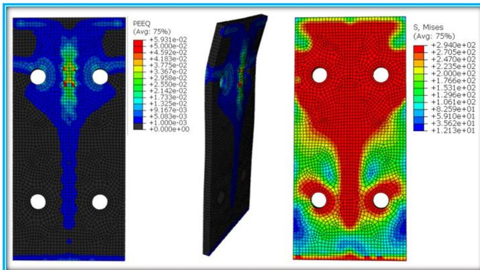
Figure 5- 15: Plastic Strains & Stress Distribution at the End Plate (ABAQUS - Ideal Plastic Model)
