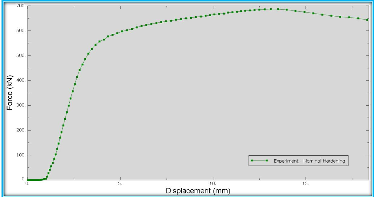
Figure 3 - 29: Experiment Joint - Force vs Displacement Curve (Nominal Hardening)
