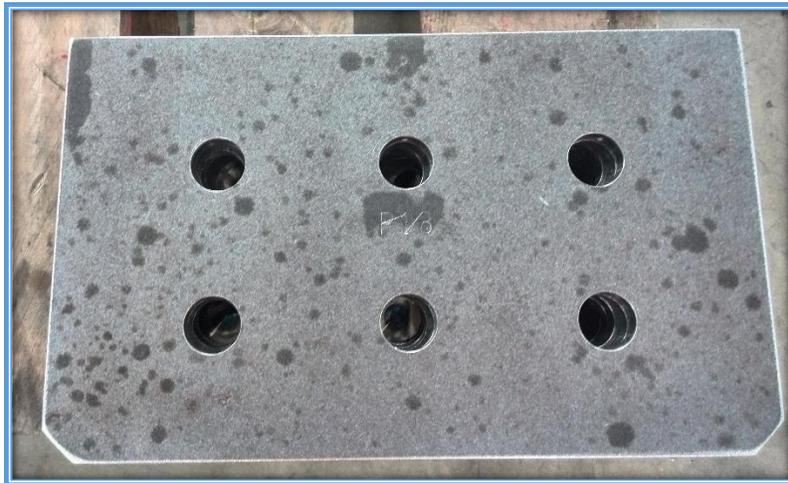
Figure 3 - 3: Fin Plate after Machining
