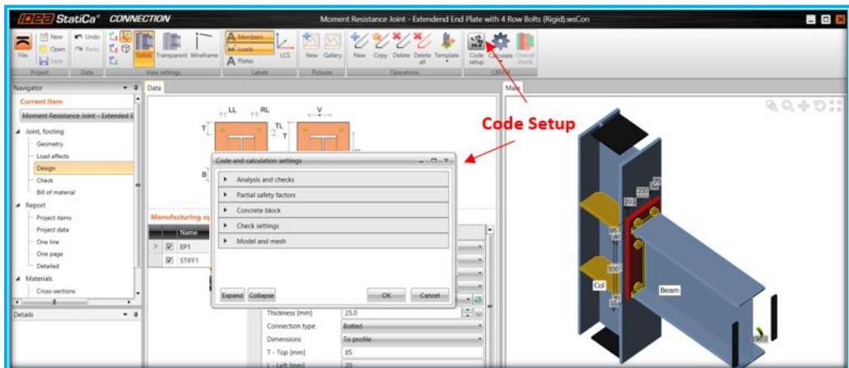
Figure A - 6: Code Setup Location
