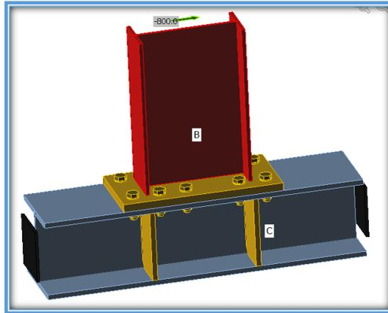
Figure 3 - 20: Beam Clamp Model in IDEA StatiCa
