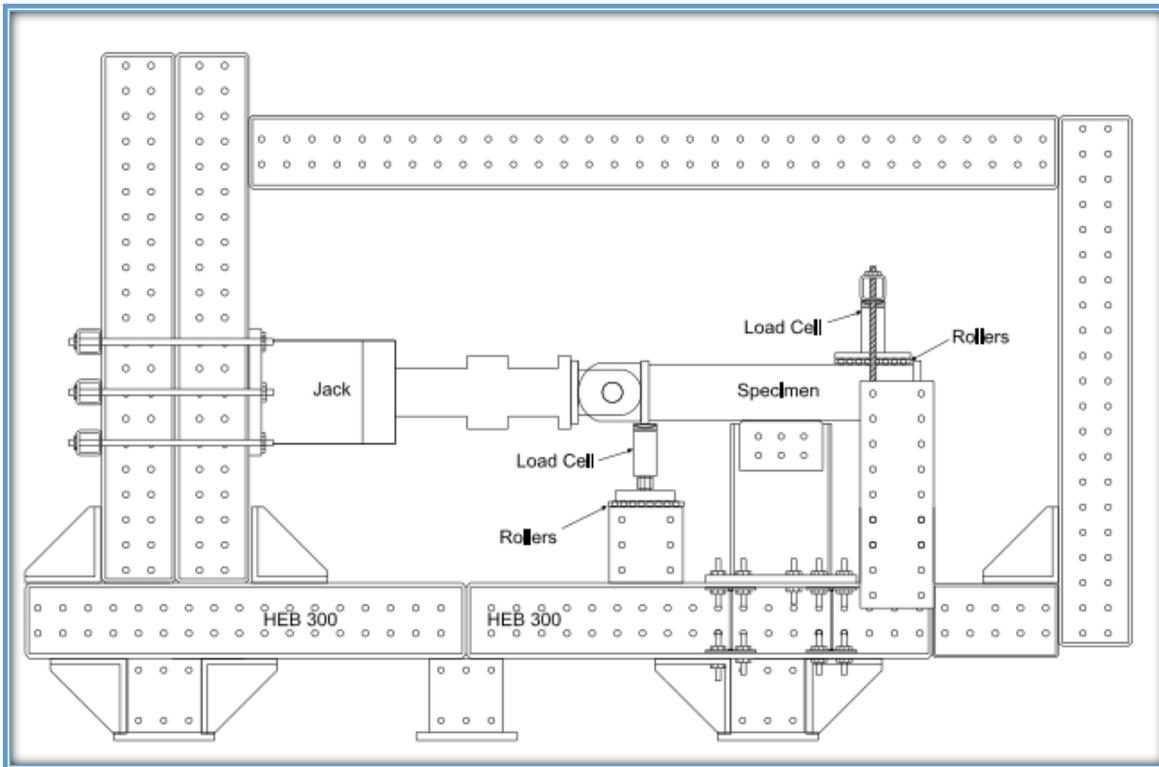
Figure 3 - 19: Frame Setup
