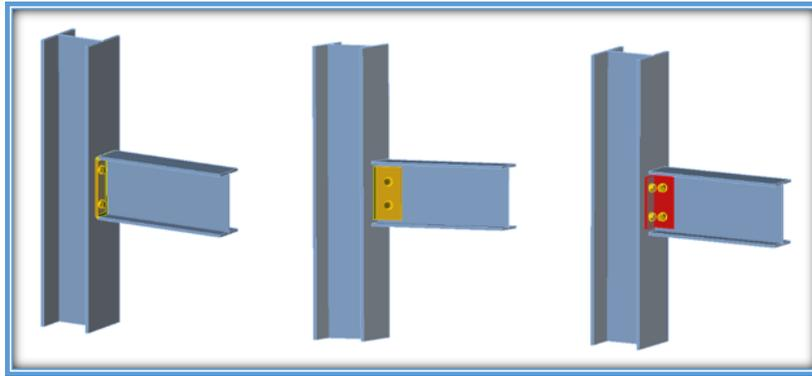
Figure 2 - 2: Types of Simple Joints
