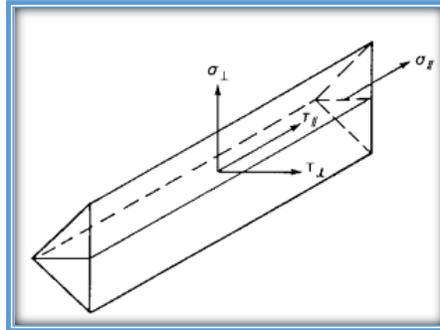
Figure 4 - 5: Stress Location at a Fillet Weld
