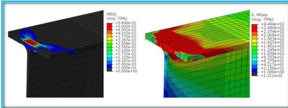
Figure 5- 23: Rigid Joint - Strain and Stress Distribution of the Beam Flange (ABAQUS - Ideal Plastic)
