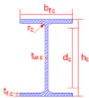
$$\begin{array}{llll} h_c := 478 \text{ mm} & r_c := 27 \text{ mm} & A_c := 33540 \text{ mm}^2 & \\ b_{f,c} := 307 \text{ mm} & d_c := 344 \text{ mm} & & \\ t_{w,c} := 21 \text{ mm} & f_{y,c} := 275 \text{ MPa} & \varepsilon_c := \sqrt{\frac{235 \text{ MPa}}{f_{y,c}}} = 0.92 & \\ t_{f,c} := 40 \text{ mm} & f_{u,c} := 360 \text{ MPa} & & \end{array}$$
