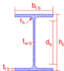
$$\begin{array}{llll} h_b := 400 \text{ mm} & r_b := 21 \text{ mm} & I_b := 23.13 \cdot 10^7 \text{ mm}^4 & \\ b_{f,b} := 180 \text{ mm} & d_b := 331 \text{ mm} & A_b := 8450 \text{ mm}^2 & \\ t_{w,b} := 8.6 \text{ mm} & f_{y,b} := 275 \text{ MPa} & \varepsilon_b := \sqrt{\frac{235 \text{ MPa}}{f_{y,b}}} = 0.92 & \\ t_{f,b} := 13.5 \text{ mm} & f_{u,b} := 360 \text{ MPa} & & \\ W_{pl,b} := 1307000 \text{ mm}^3 & & & \end{array}$$
