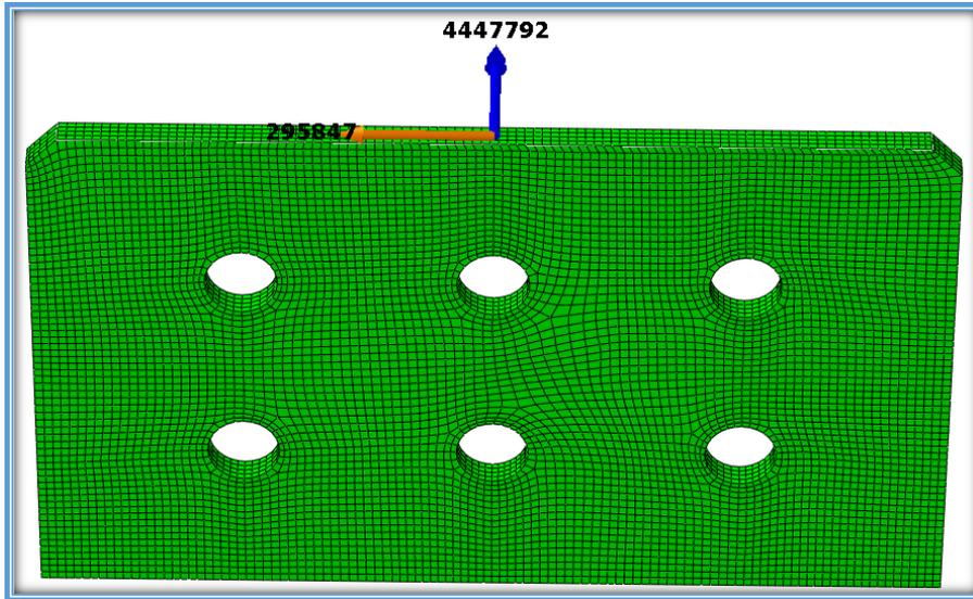
Figure 3 - 37: Shear and Bending Moment at the Fin Plate
