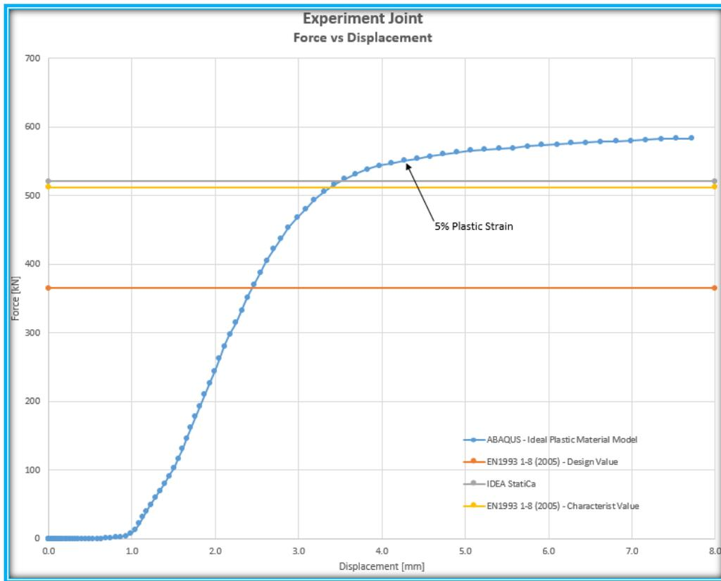
Figure 3 - 30: Experiment Joint Predictions
