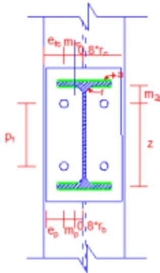
$$e_{fc} := 103.5 \text{ mm} \quad e_p := 40 \text{ mm} \quad p_1 := 200 \text{ mm}$$
