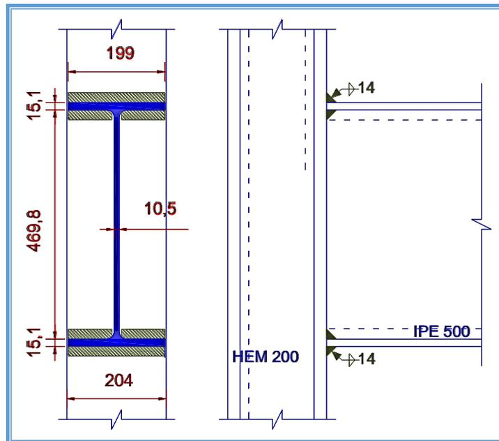
Figure 5- 19: Rigid Joint Detail (T106-004)
