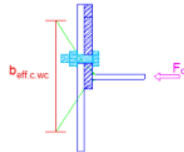
$$\omega := \frac{1}{\sqrt{1 + 1.3 \left( \frac{b_{eff,c,wc} \cdot t_{w,c}}{A_{v,c}} \right)^2}} = 0.79$$
