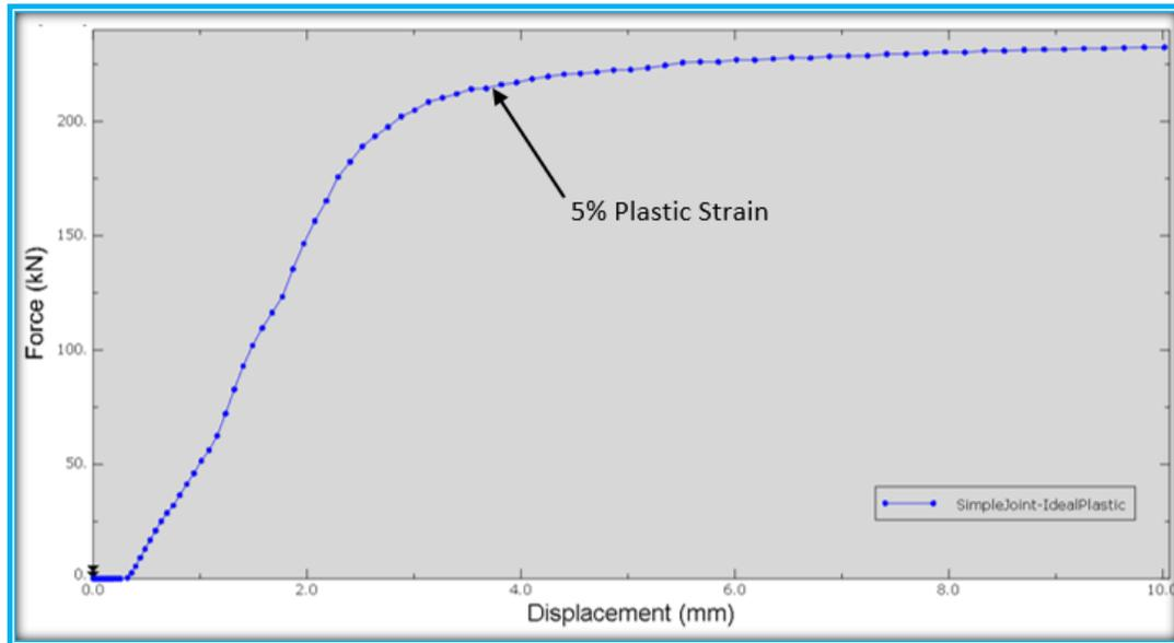
Figure 5- 8: Simple Joint - Force vs Displacement Curve (ABAQUS)
