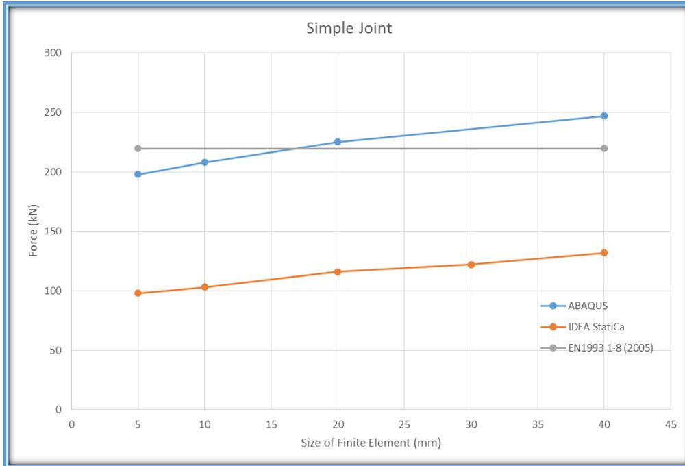
Figure 5- 10: Finite Element Size Effect
