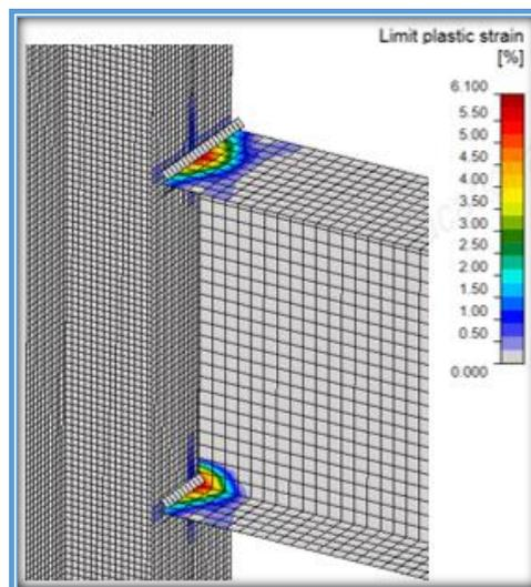
Figure 5- 22: Rigid Joint - Plastic Strain Distribution (IDEA StatiCa)
