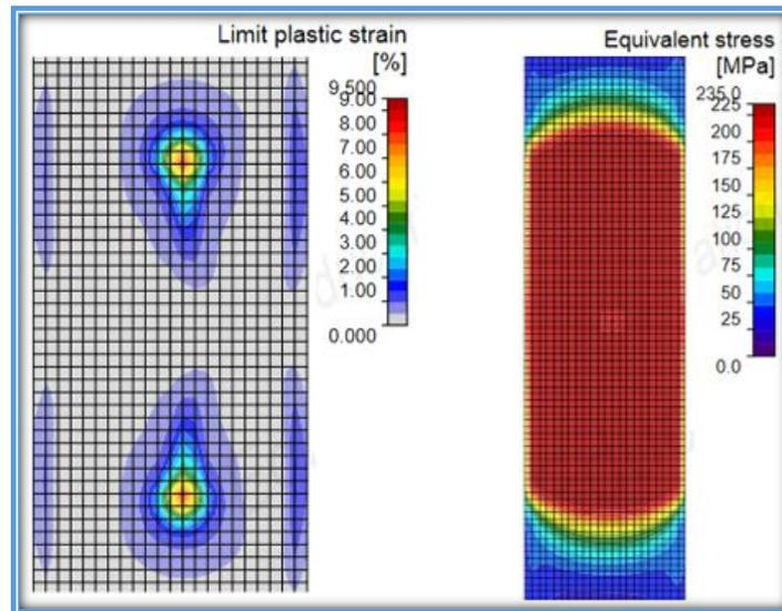
Figure 5- 4: Simple Joint - Strain/Stress distribution at the Column Web
