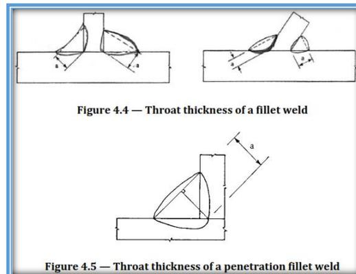
Figure 4 - 6: Weld Throat thickness ( $a$ )
