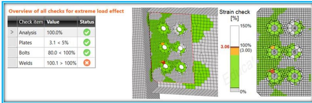
Figure 3 - 25: Experiment Joint - Results and Plastic Strain Distribution (IDEA StatiCa)
