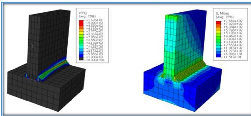
Figure 4 - 12 Stress/Strain Distribution in the Shear Loaded Weld
