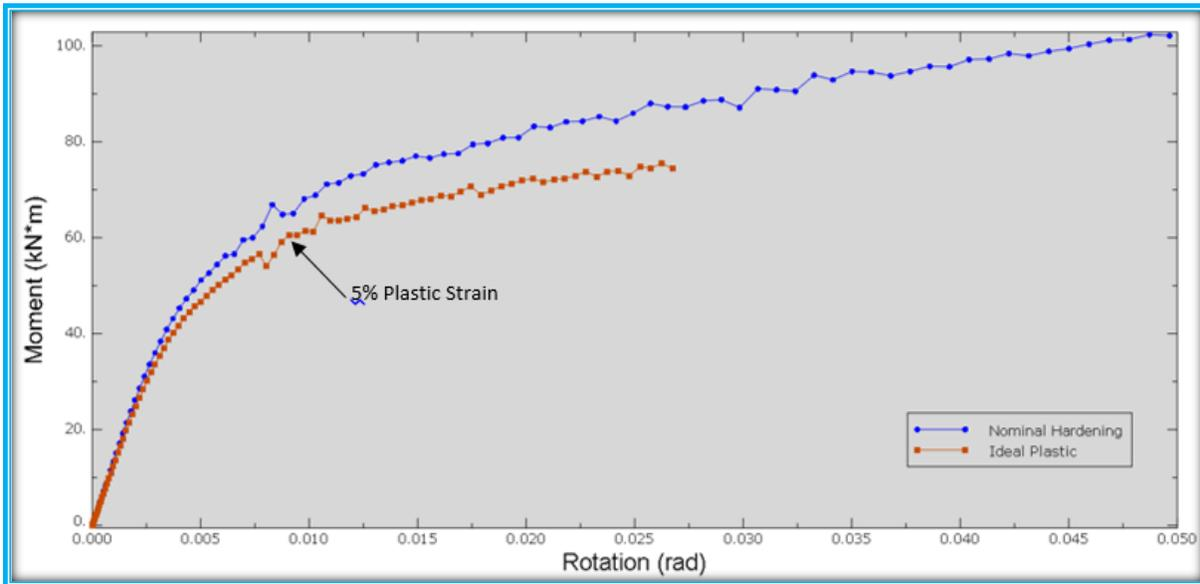
Figure 5- 17: Semi-Rigid Joint – Moment vs. Rotation Curves (ABAQUS)
