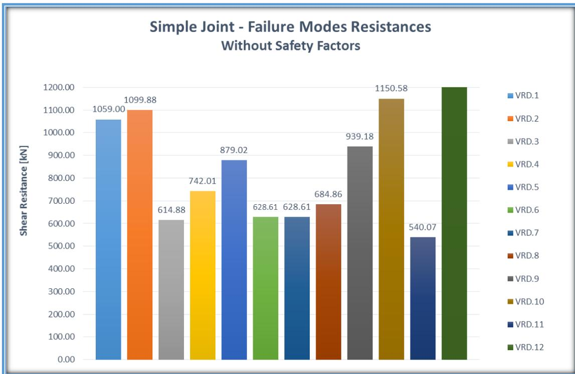
Figure 3 - 24: Experiment Joint - Hand Calculation Results
