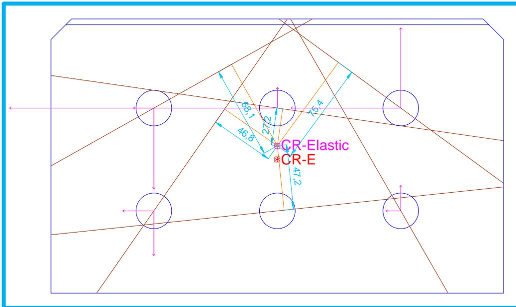
Figure 3 - 36: Perpendicular Distance between the Resultant and the Center of Rotation
