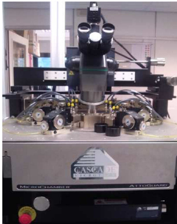
CASCADE MICROTECH Probe Station 34 Used for: Transistor measurements of chapter 5
