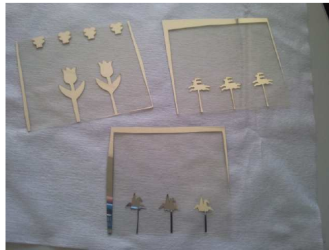
Figure 8.3: The plastic substrate with a layer of 300 nm aluminium shapes deposited on top by electron beam evaporation
