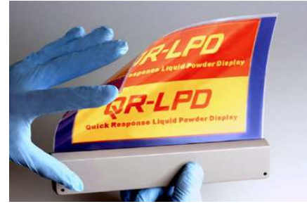
Figure 4.5: QR-LPD developed by Bridgestone [13]
