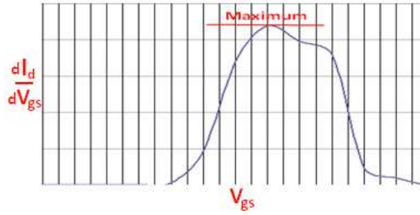
Figure 5.1: Computing mobility from the dI_d/dV_{GS} graph of an NMOS transistor.
