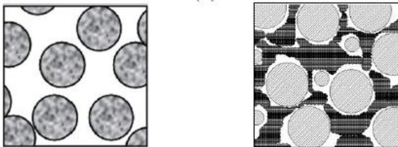
Figure 2.3: Schematized packing densities for a sand-silt mixture, without (left panel) and with (right panel) clay particles (Jacobs, 2011).
