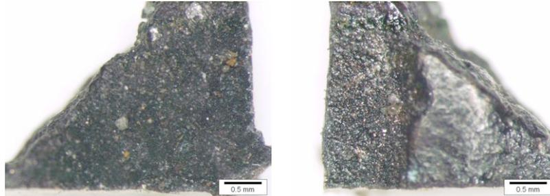
Fig. 23: Morphology on the inner (left) and outer (right) surface of sample BH76#3 from the Tongeren axe. The casting seam is visible at the outer surface (right). Optical micrographs.
