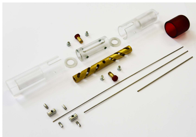
Figure 7. Prototype Biopsy Needle showing all the parts.
