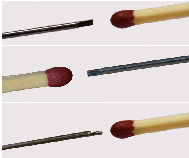
Figure 8. Prototype Biopsy Needle Tip Designs. Top—beveled blade design. Middle—straight blade design. Bottom—reverse-beveled blade design. The match is shown for scale purposes.
