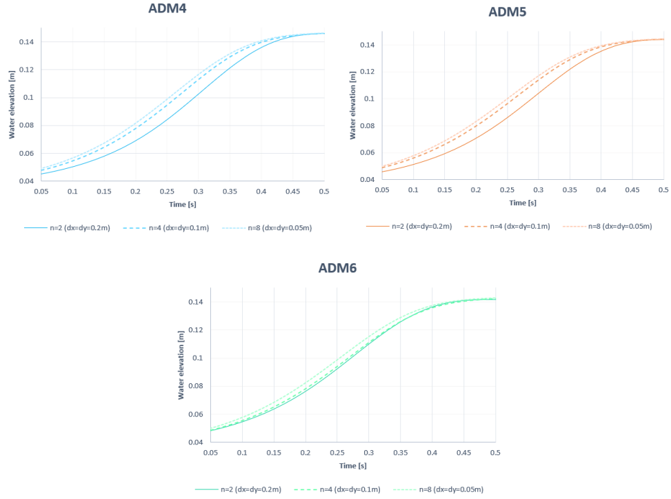
Figure B.1: Comparison of 3 different mesh sizes for the optimal 2D space resolution.
