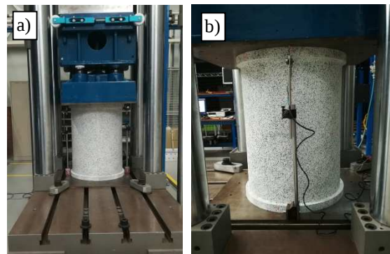
Figure 4. MTS 3500 kN servo-hydraulic test machine: a) front view; b) side view
