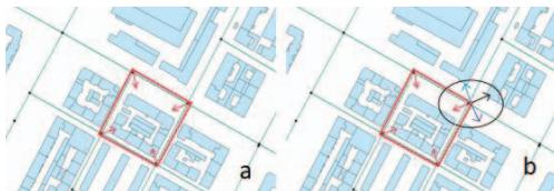
Fig. 4. (a) Water demand  $Q_{\text{demand},j,w}$  within a mesh element  $w$  in district  $j$ , (b) Water demand at node  $i$ .
