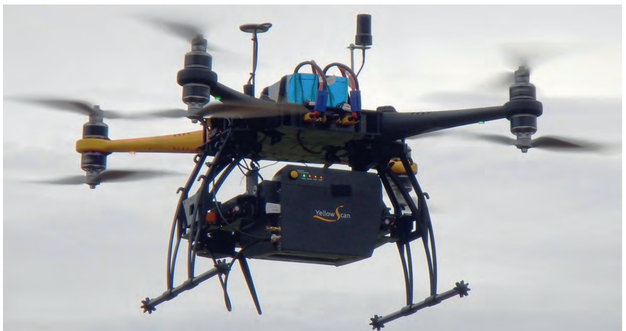
▲ Figure 7, The YellowScan Mapper lightweight Lidar system in operation.
