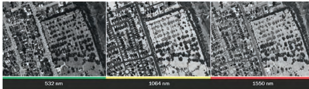
▲ Figure 3, Multispectral images created from a Titan airborne Lidar system manufactured by Teledyne Optech.
