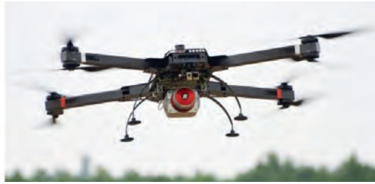
▲ Figure 6, The RIEGL VUX-1 Lidar system is small enough to be carried by a UAS.
