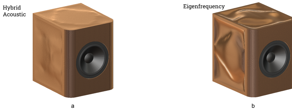
Figure 6.18: Render of the final cabinets of the hybrid acoustic (a) and eigenfrequency optimisation (b).
