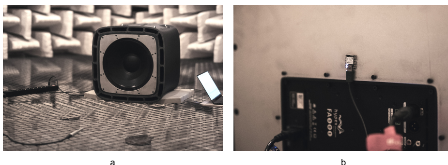
Figure 5.2: Setup of the Reflex Sub within the Anechoic chamber (a) and the IMU mounted to the rear panel of the subwoofer (b).
