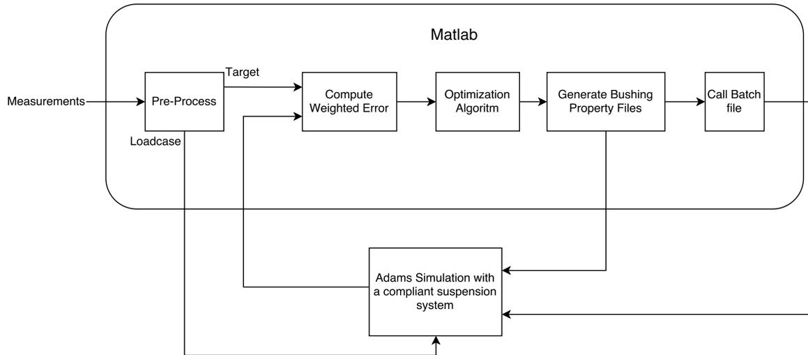
**Figure 4-2:** Diagram of the SIL architecture.
