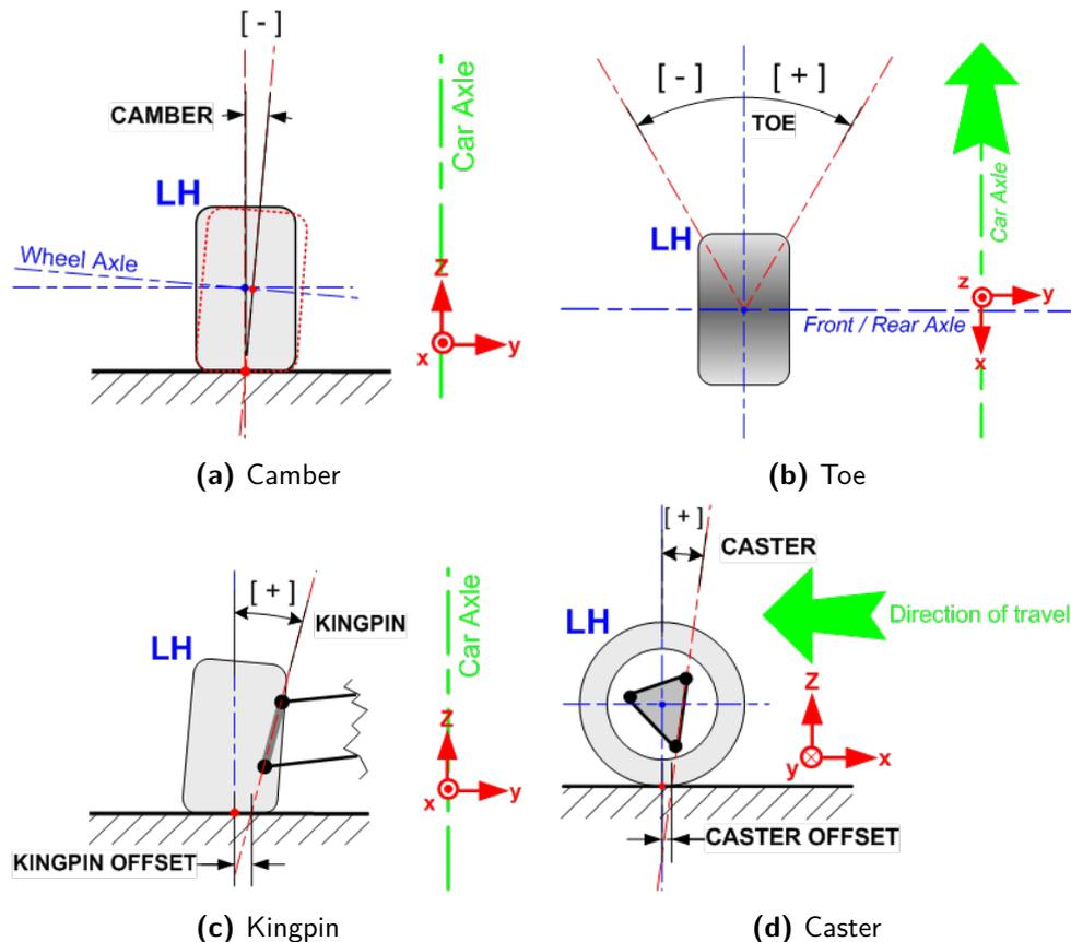
Figure 2-2: Definition of the main geometric metrics [21].
