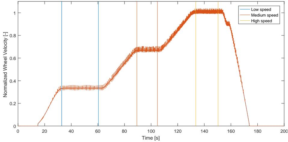
**Figure 3-1:** Speed profile during the test, with the selection marked.
