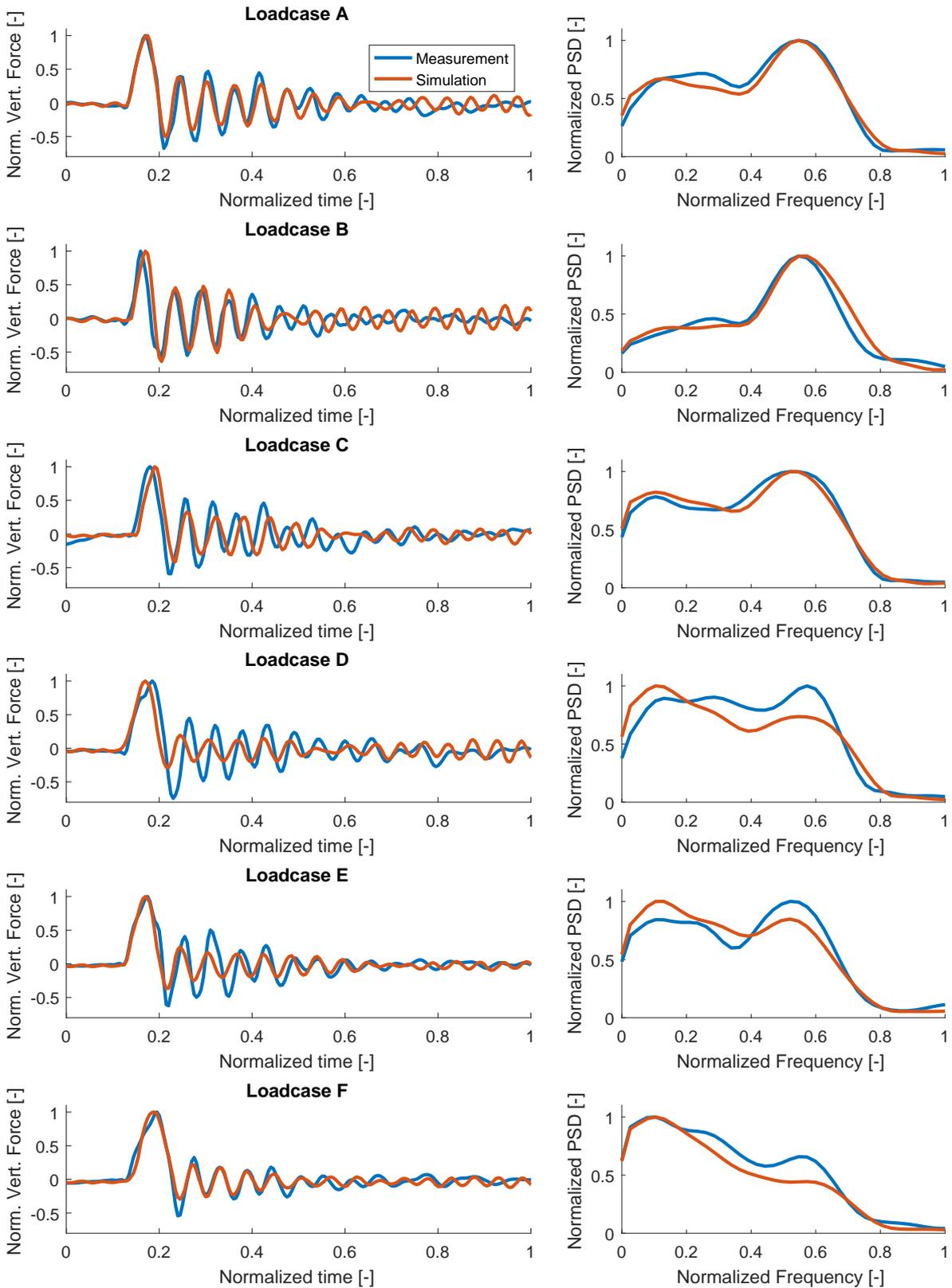
**Figure 3-7:** A compare of the FTire simulation to the measurement.
