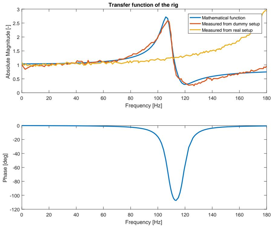
**Figure 3-5:** Frequency Response of the Rig compared to the found Mathematical Function.
