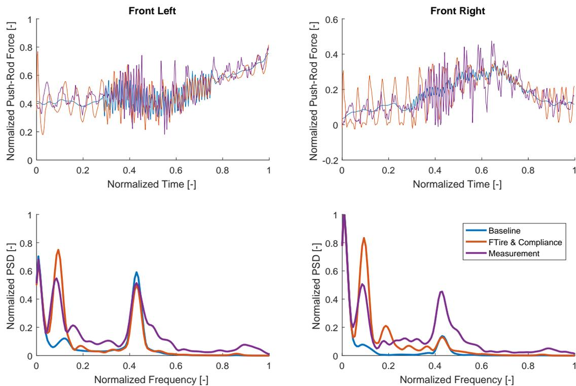
**Figure 5-6:** Plots of the baseline and final model compared to Track Measurements.
