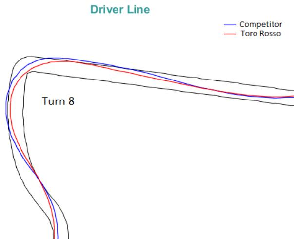
**Figure 1-2:** Difference in driving line at turn 8 shown on the track map.
