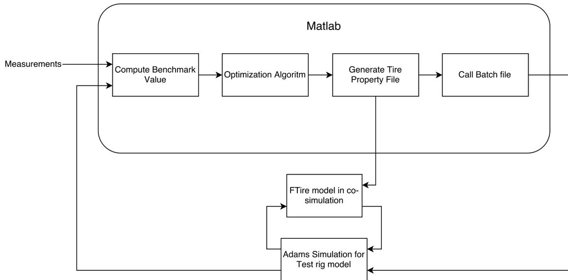
**Figure 3-6:** Diagram of the SIL architecture.
