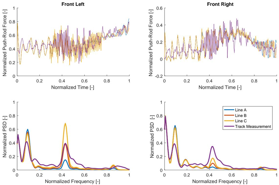
Figure 5-5: Sensitivity on the Driving line.
