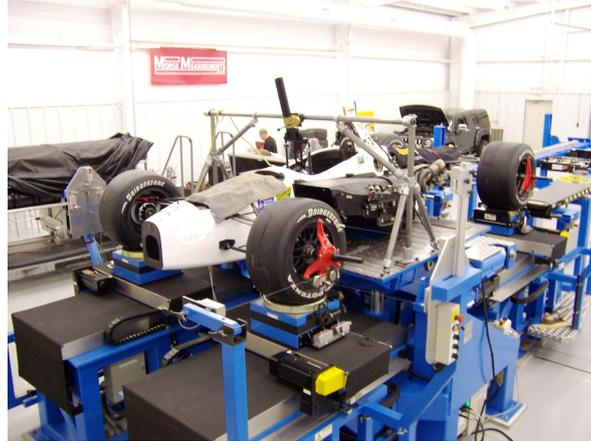
**Figure 2-3:** A racing car on a K&C machine [24].
