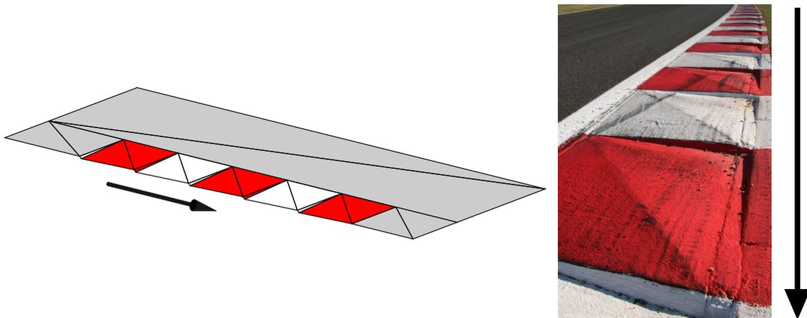
**Figure 5-3:** Geometry of the Kerbstone, on the left the 3D model, on the right a photo [33].
