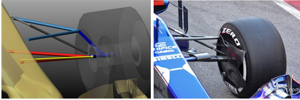
**Figure 4-1:** Image of the outboard suspension (Left: Screenshot MSC.Adams, Right: Photo [3]).
