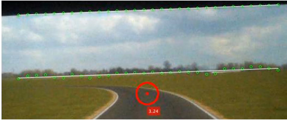
Figure C.2: Example of a recorded baseline frame, showing the transition points (green) regressions of the scene edge and the horizon (white lines), as well as the gaze position (red).
