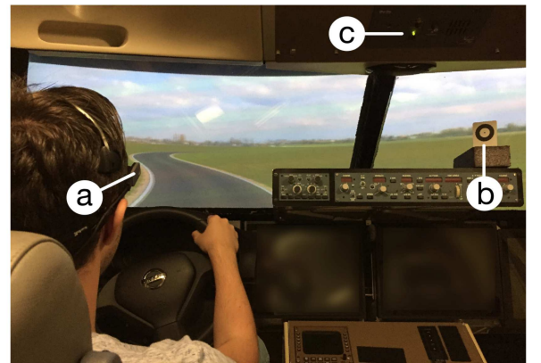
Fig. 4: Picture of a participant performing the baseline condition, illustrating the experiment setup. Component [a] is the eye tracker, [b] is the eye tracker calibration point and [c] is the reference LED light.
