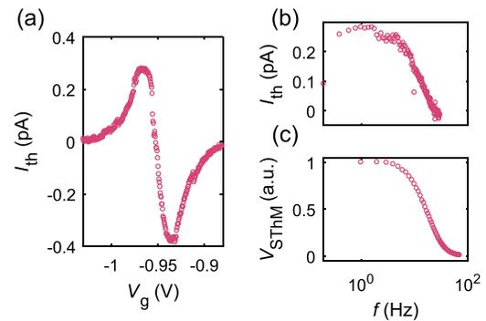
**FIG. 4.** (a) AC thermocurrent ( $f = 3$  Hz,  $I_{heater} = 0.1$  mA,  $P_{heater} = 26$   $\mu$ W) as a function of gate voltage. (b) Thermocurrent at  $V_g = -0.965$  V as a function of modulation frequency of the sample heater. (c) SThM signal on the drain (hot) contact as a function of modulation frequency of the sample heater.
