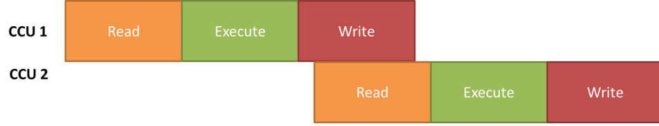
Figure 3.10: Pipelined sequential execution with TLB Support
