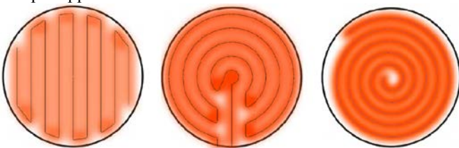
Fig. 10. Three layout concepts: the spiral concept shows the most uniform heat distribution without hotspots.
