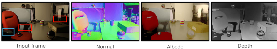
Figure 2.21: Reconstruction results of the scene parameters for a complex, large scale real-world data set of an office work space. While a few artifacts occur in areas which are barely lit (red), feature very dark materials (blue) or interreflection (the camera-facing side of the cardboard), most parts are truthfully reconstructed by our method.
