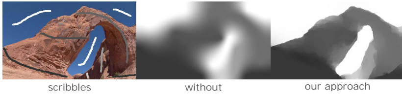
Figure 3.4: Depth estimation from scribbles. Scribble input (left), only using the scribble input results in a smooth depth map lacking discontinuities (middle), by involving the input image gradients, the depth propagation is improved (right). (Image source: www.pixabay.com )
