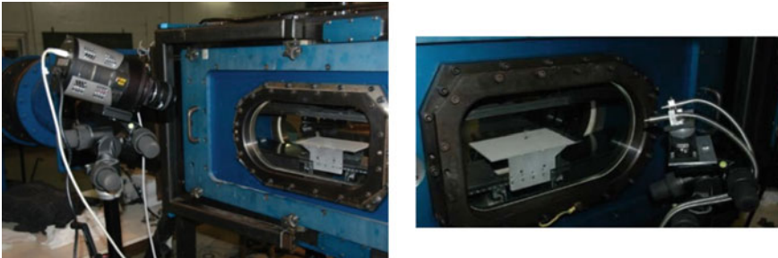
Fig. 24 Temperature Sensitive Paint arrangement near the test set-up of the S8Ch wind tunnel
