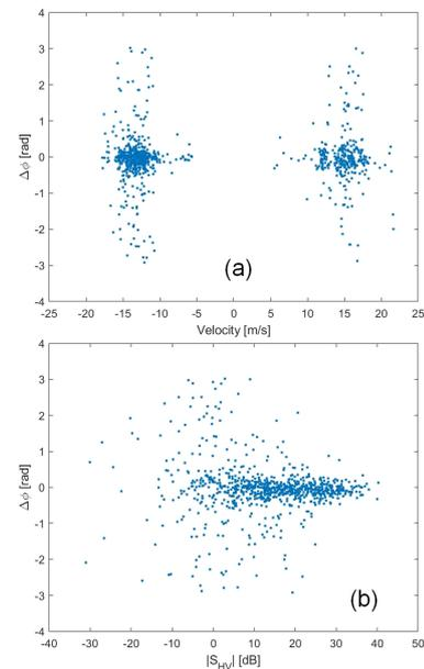
Fig. 7. Compensation results on the phase difference between the PSM elements  $S_{HV}$  and  $S_{VH}$  in case of unambiguous Doppler velocity: (a) the compensated phase difference; (b) the compensated phase difference w.r.t. signal amplitude
