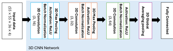
Fig. 7: Structure of the 3D CNN network. Input data is represented as 4-D tensors with intensity values plus 3 components of velocity vectors. The size of convolutional layers is described as [CNN kernel size, number of channels].
