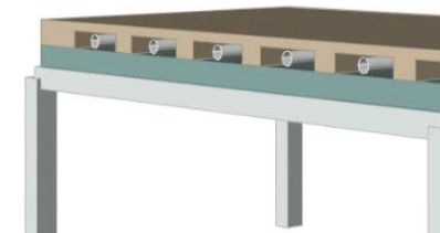
Services in raised floor
