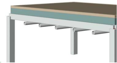
Ducts below beams
