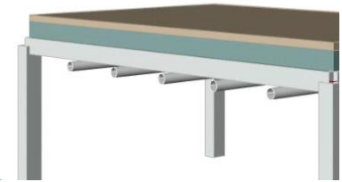
Ducts below beams
