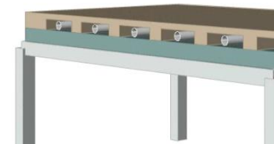
Services in raised floor
