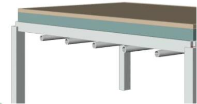
Ducts below beams
