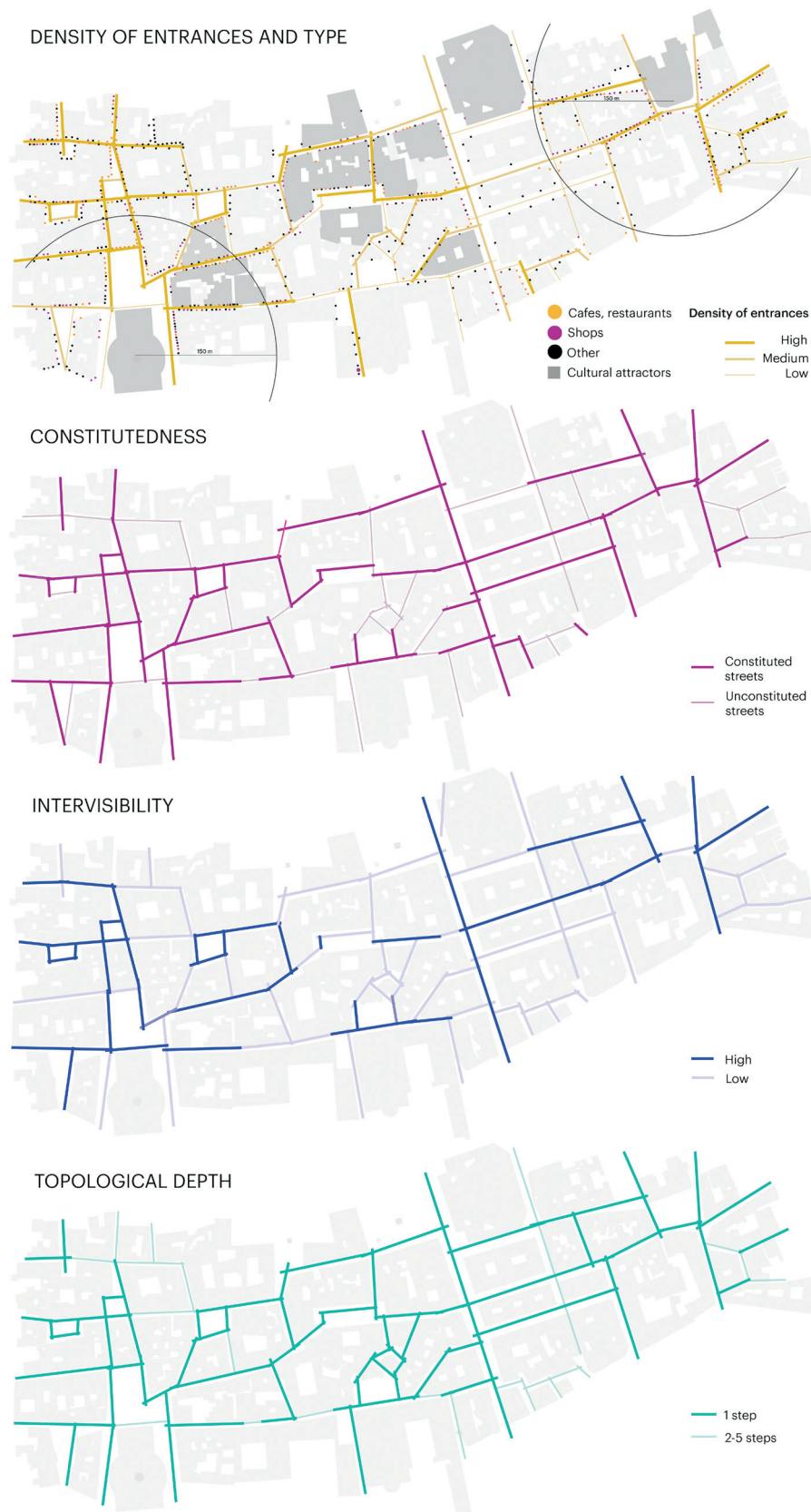
Figure 10. Micro-spatial parameters: density of entrances and type, intervisibility, constitutedness, topological depth.
