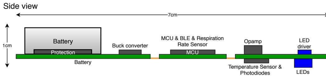
Figure 5.2: Side view of physical prototype
