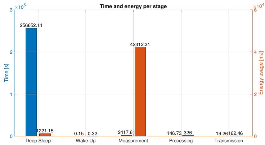
Figure D.7: Distribution of time and energy over the different stages in the full system simulation of the sensor patch.
