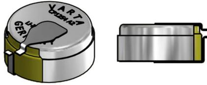
Figure 4.5: Possible battery mounting [39].
