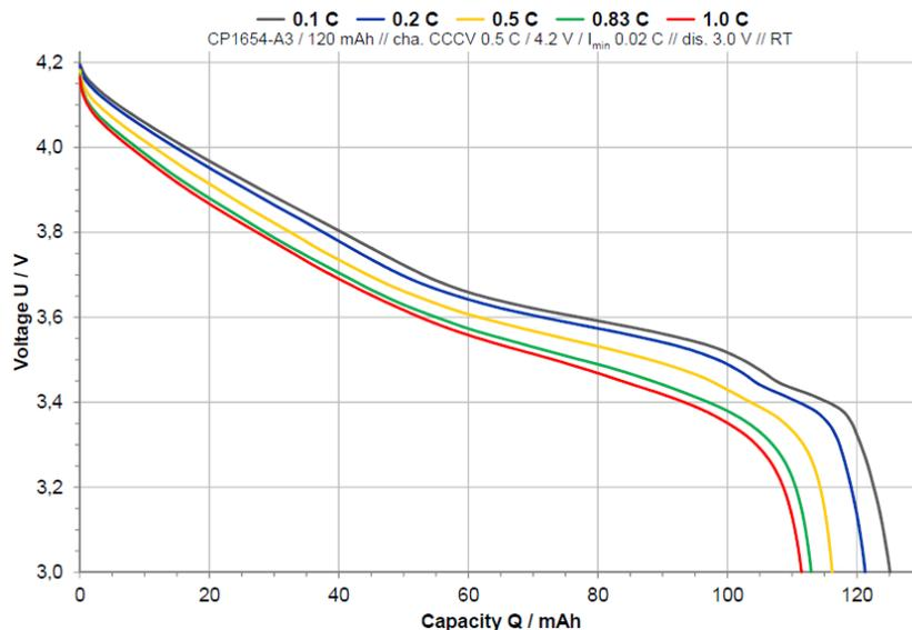
Figure 3.7: CP1654A3 - Discharge characteristics at various C-rates
