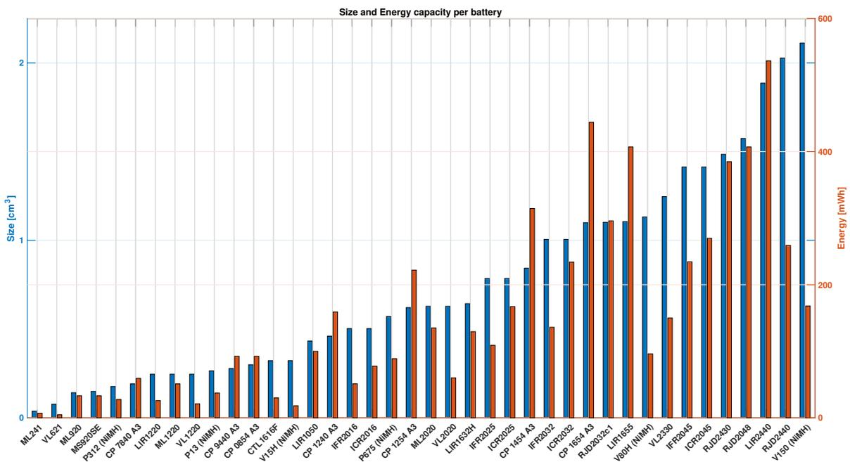
Figure C.1: Bargraph of the size and energy capacity of all the batteries
