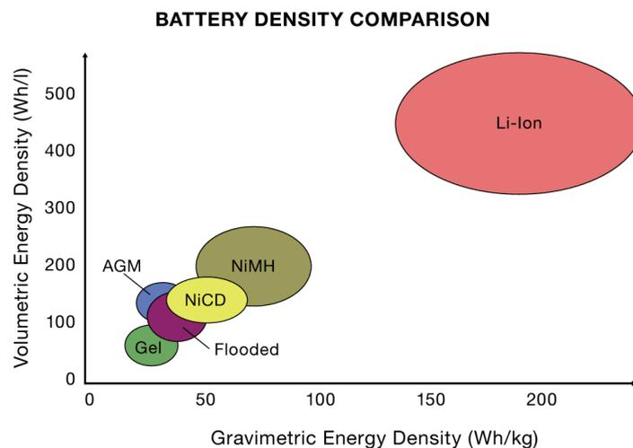
Figure 3.4: This is a battery density comparison from the book Off Grid Solar. [20]
