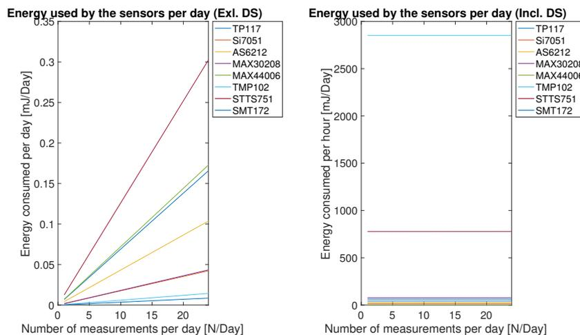
Figure 4.2: Plot of the energy consumed per sensor per day, depending on number of measurements.
