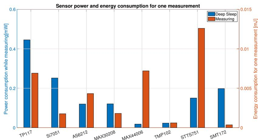
Figure 4.1: Bargraph of the power drawn and energy usage for each sensor during one measurement.
