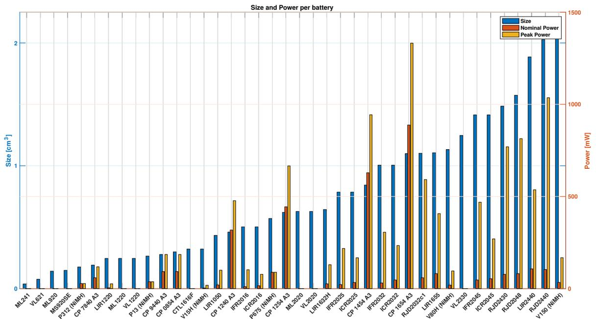
Figure C.3: Bargraph of the size and nominal&maximum power of all the batteries
