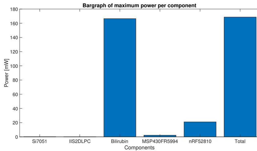
Figure D.8: Maximum power drawn per component in the full system simulation.
