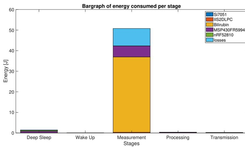
Figure D.6: Energy usage per stage divided per component in the full system simulation.
