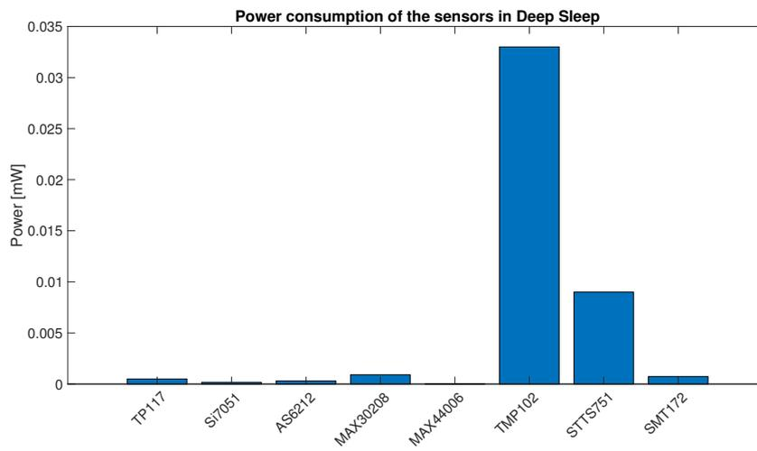
Figure D.1: Bargraph of the power consumption of sensors in deep sleep.
