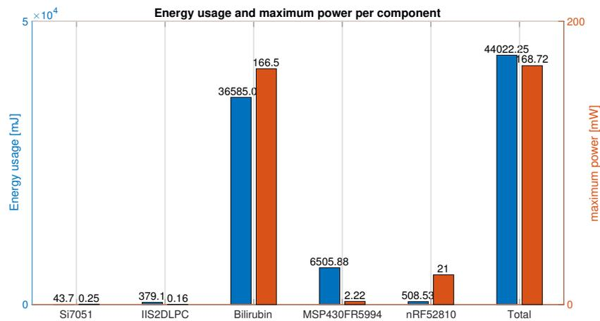
Figure 4.4: Energy usage and maximum power per component in the full system simulation without losses.
