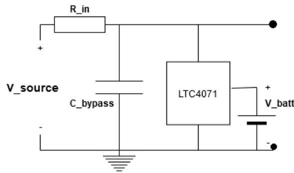
Figure 4.8: Lithium-ion Battery Charger
