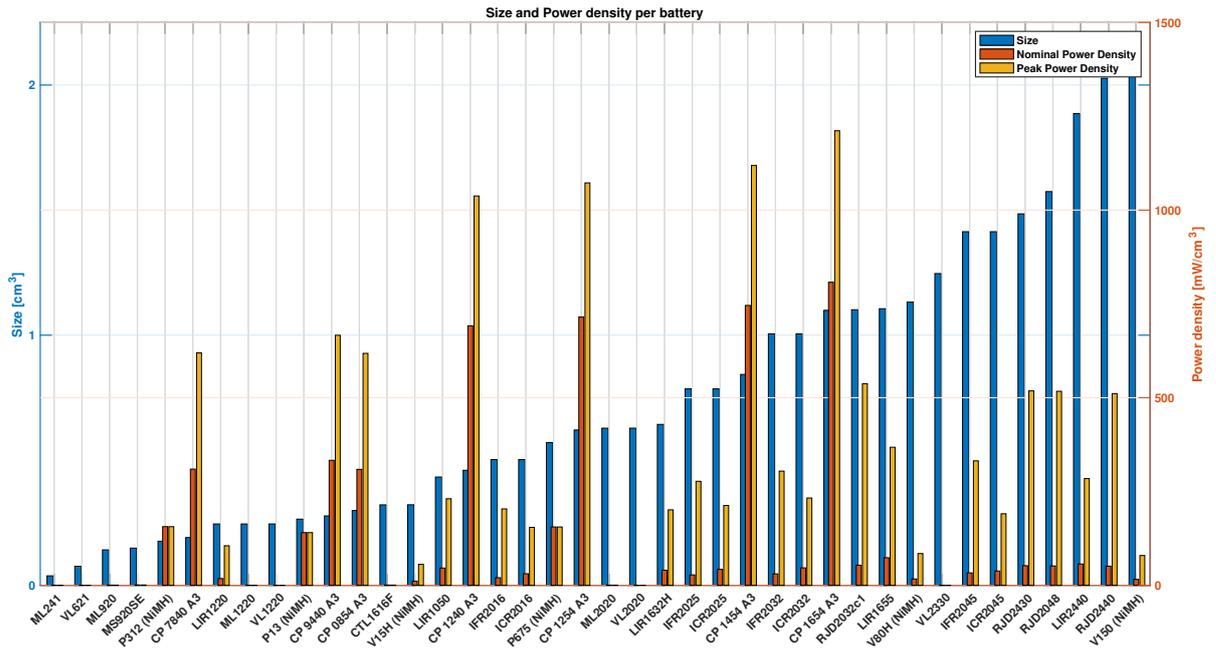
Figure C.2: Bargraph of the size and power density of all the batteries
