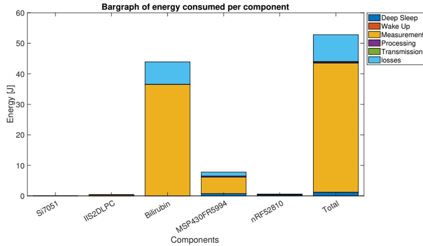
Figure 4.3: Energy usage per component divided per stage in the full system simulation.
