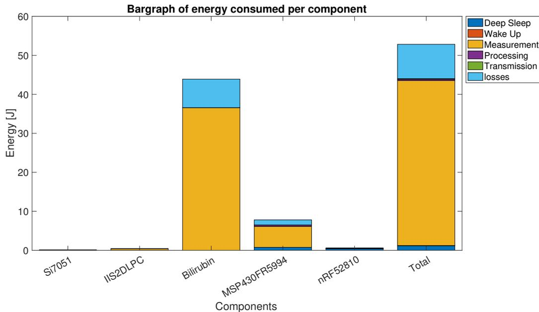
Figure 5.4: Energy usage per component divided per stage in the full system simulation.
