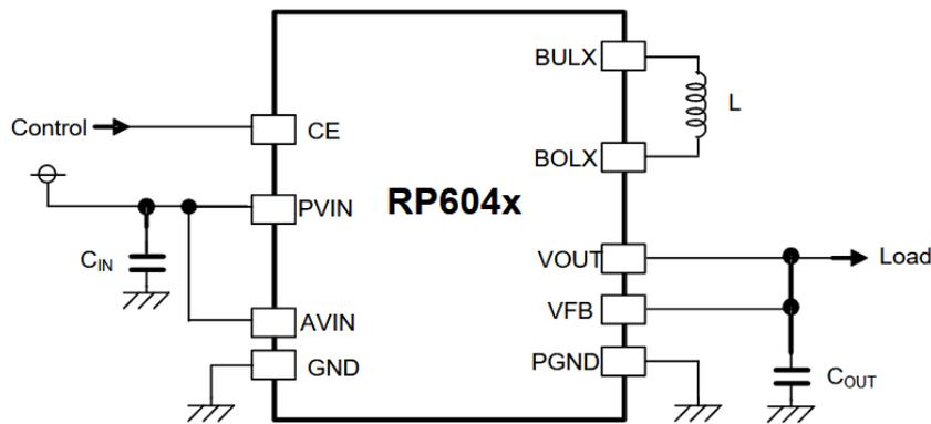
Figure 4.7: RP60437 Schematic
