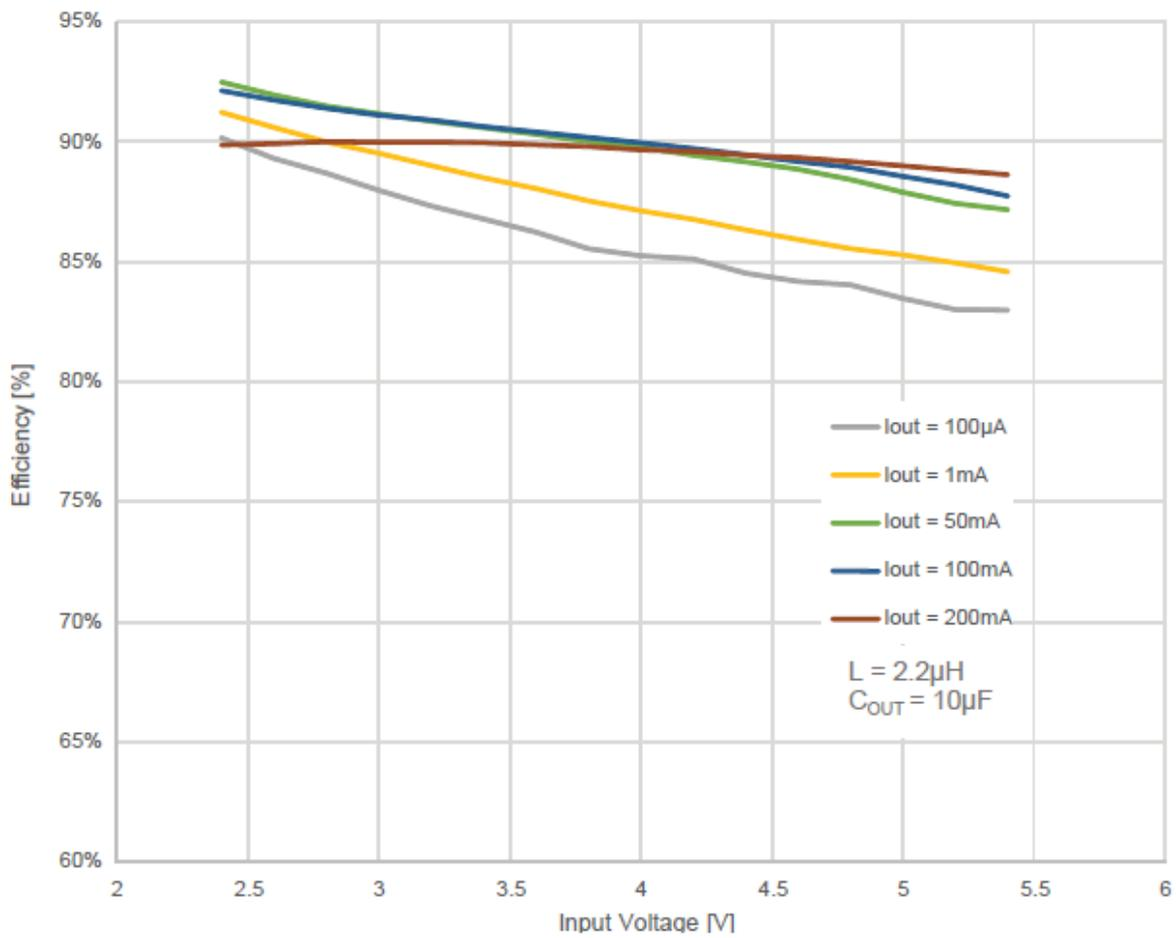
Figure E.1: Buck converter: Efficiency vs. Input voltage, Output voltage = 1.8V
