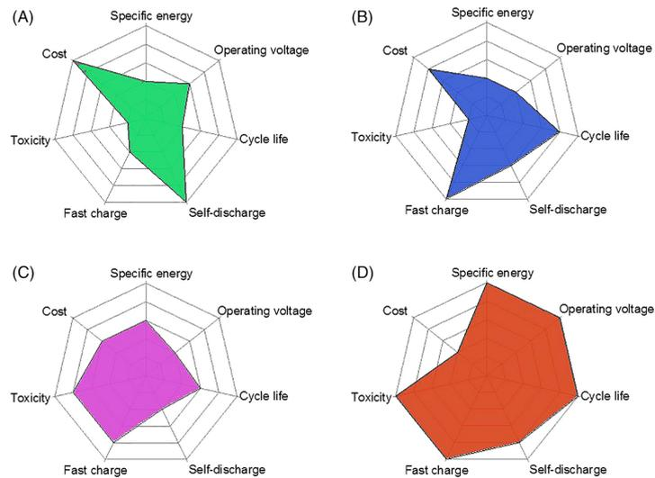
Figure 3.3: Performance comparison of A, lead-acid, B, Ni-Cd, C, Ni-MH, and D, Li-ion batteries. [15]
