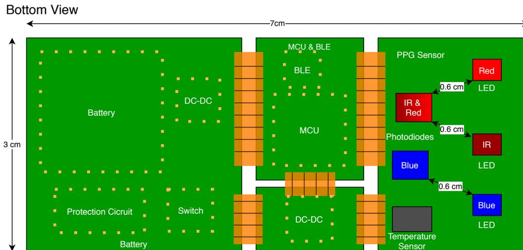
Figure 5.3: Bottom view of physical prototype
