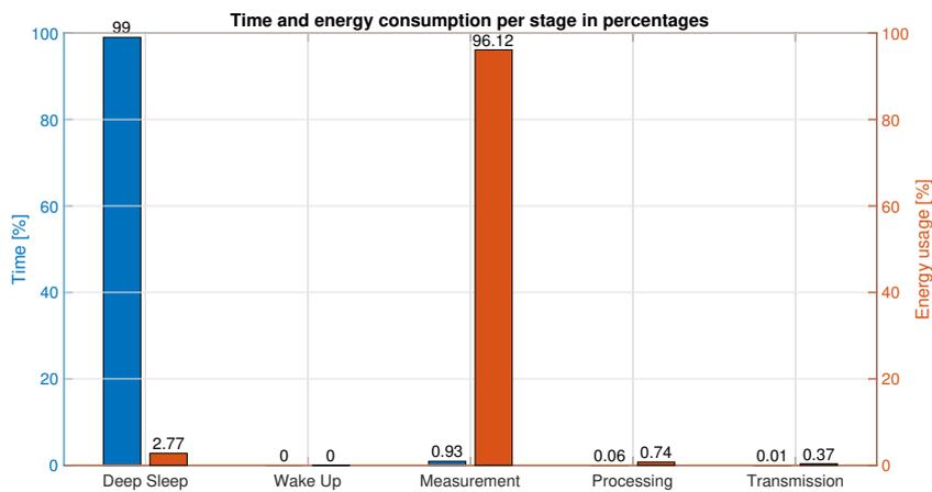
Figure D.5: Distribution of time and energy (in percentages) over the different stages in the full system simulation of the sensor patch.
