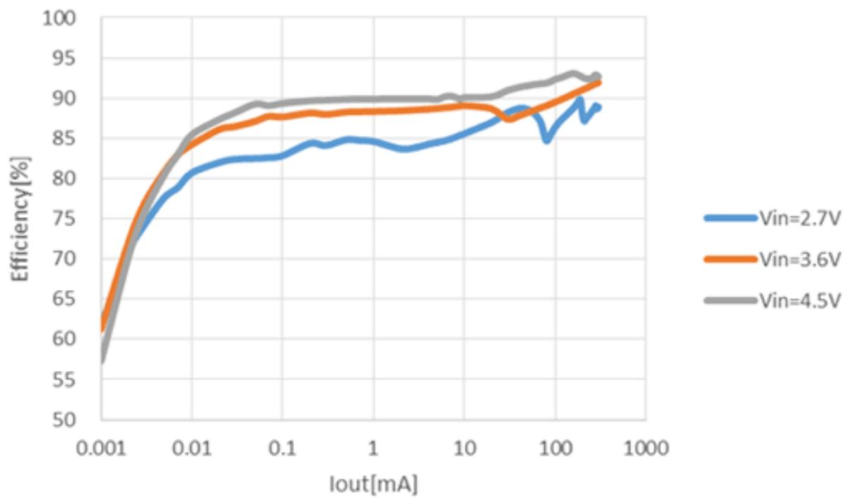
Figure E.2: Buck-boost converter: Efficiency vs. Input voltage, Output voltage = 5.0V
