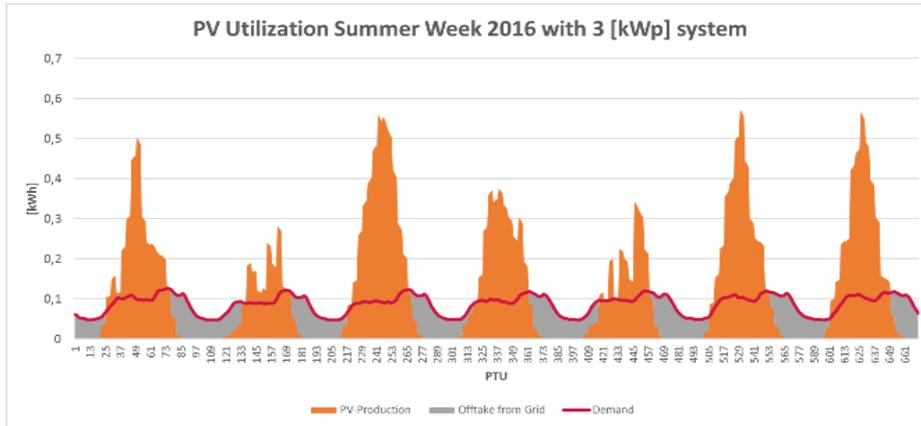
Figure 26: PV Utilization Summer Week 2016 with 3 [kWp] PV-system
