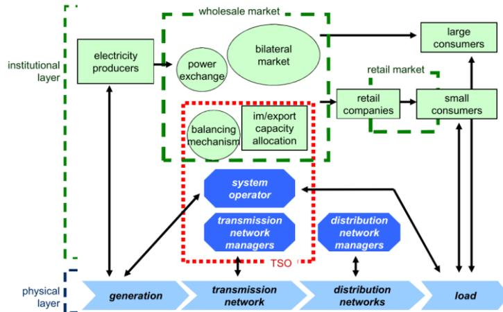
Figure 5: Dutch power system (de Vries et al., 2016)
