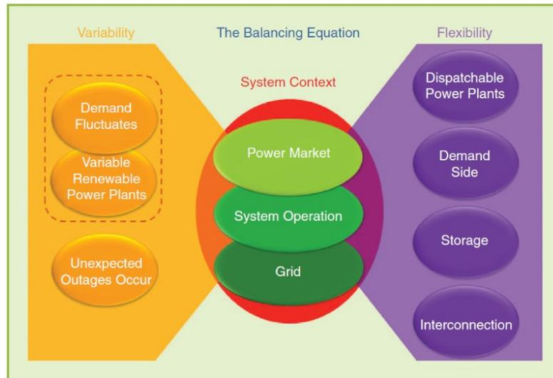
Figure 1: Flexibility needs, sources and enablers (Holtinen et al., 2013)
