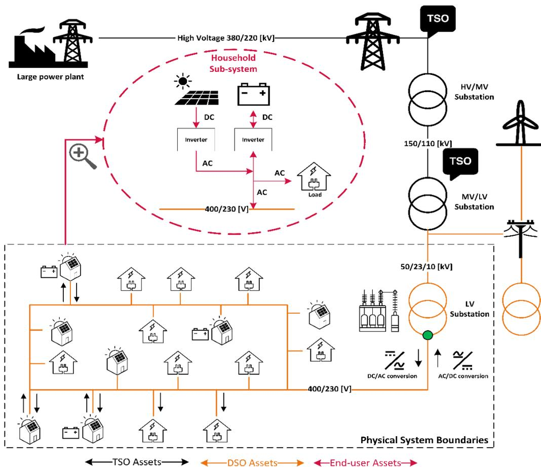
Figure 6: Physical System Diagram
