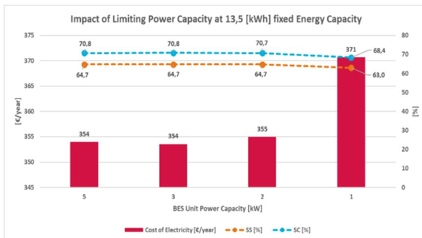
Figure 35: Output Indicators when Limiting Power Capacity
