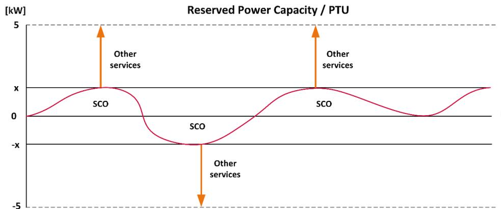
Figure 37: Potential Distribution of BES unit Power Output
