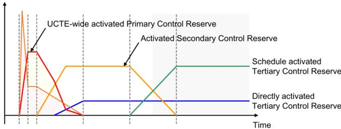
Figure 7: Principle frequency deviation and subsequent activation of reserves (ENTSO-E, 2009)
