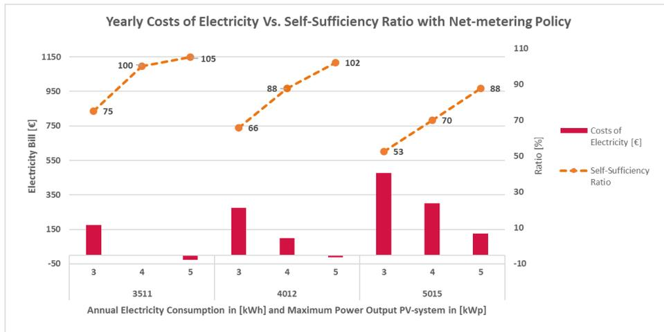
Figure 24: Yearly Costs of Electricity and Self-Sufficiency Ratio with Net-metering Policy
