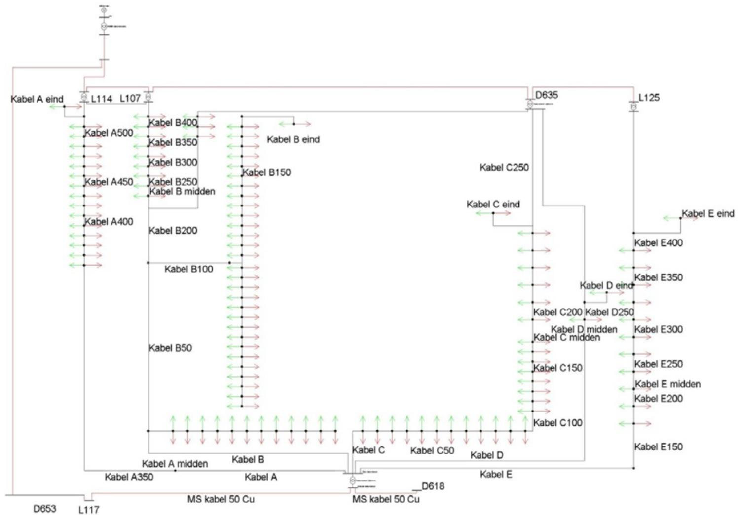
Figure 17: Meshed network structure LV distribution grid of Kijkduin
