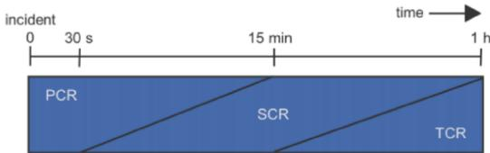
Figure 8: PCR, SCR and TCR with activation times after the incident
